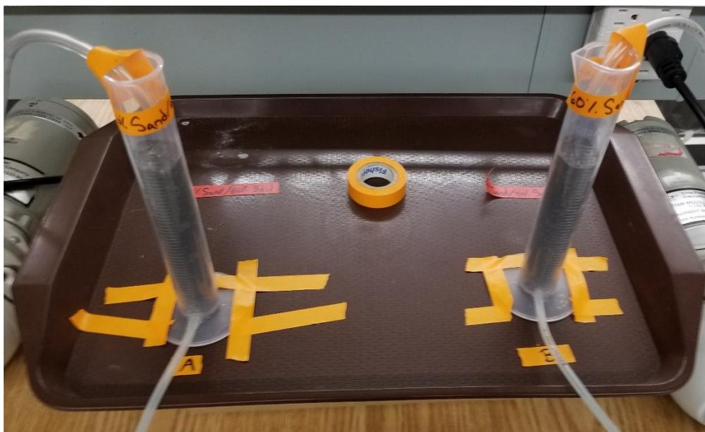
Figure 19: Set up for small columns for phosphate adsorption capacity analysis of soil media "A" and "B".
