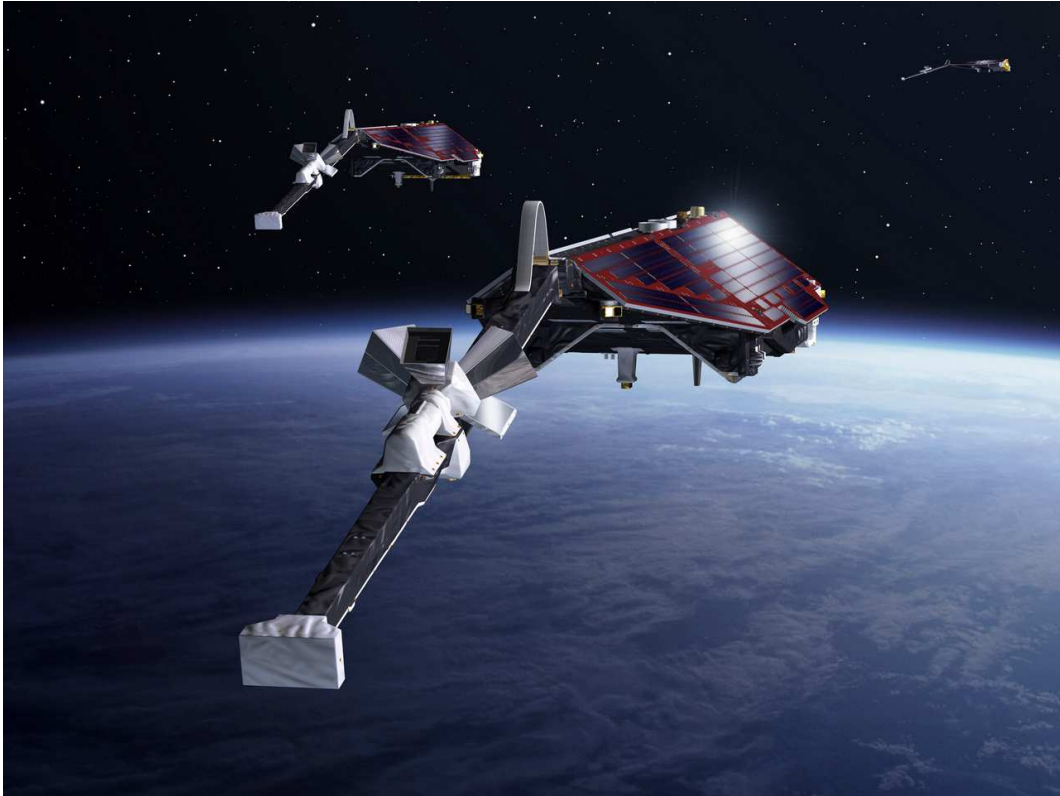
Figure 1.5: An artist's view of the three Swarm satellites in orbits. Two of the satellites are flying side by side at initial altitude of 460 km, whereas the third is orbiting at an altitude of 530 km. All three satellites have quasi-polar circular orbits. The image is reprinted with permission from the ESA website.
