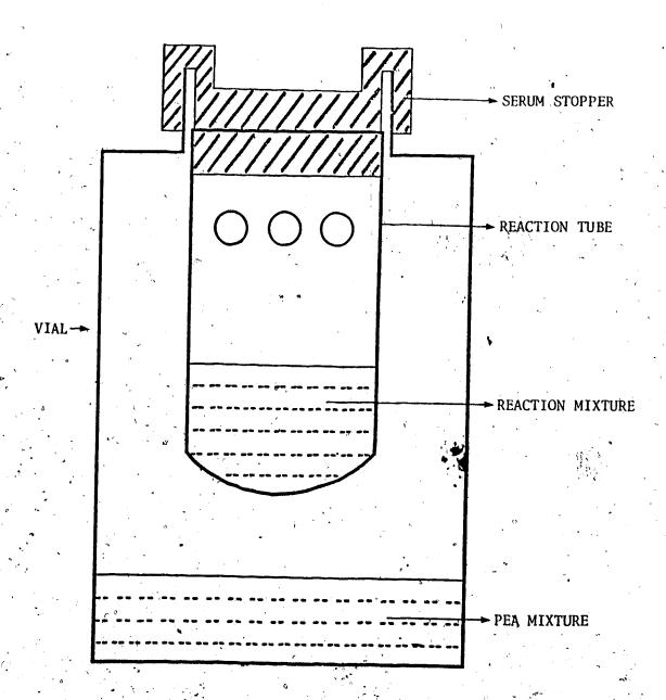
was allowed for a minimum of 2 hr at room temperature and the gas was trapped by 1 ml of a solution containing phenylethylamine (PEA)-methanol-toluene (1:1:2 by volume) in the bottom of the scintillation vial.
