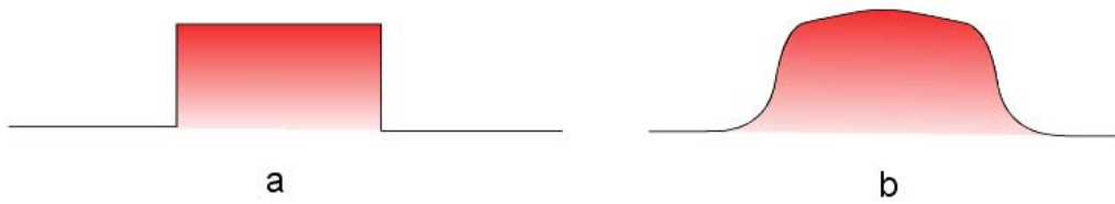
Figure 4-24 Illustration of a), a perfect top-hat profile and b), the approximate top-hat from truncating the Gaussian beam used in our experiments.
