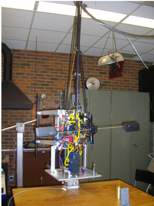
**Figure 3.4:** *Helicopter mounted for roll moment estimation. Full view.*
