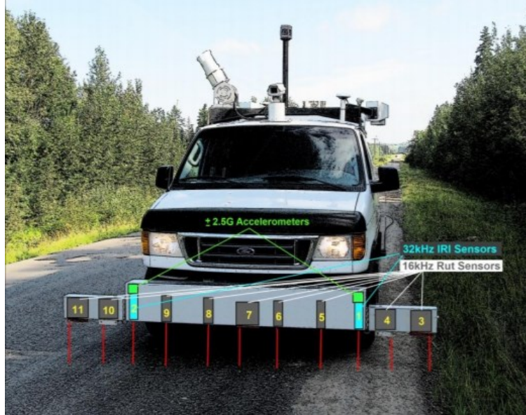
Figure 1.1. PSP-7000 survey vehicle [12]
