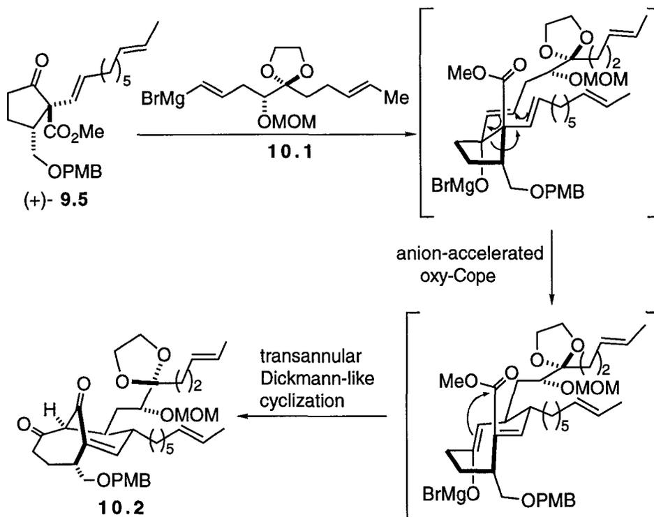
**Scheme 10.** Oxy-Cope rearrangement and transannular Dieckmann cyclization.
