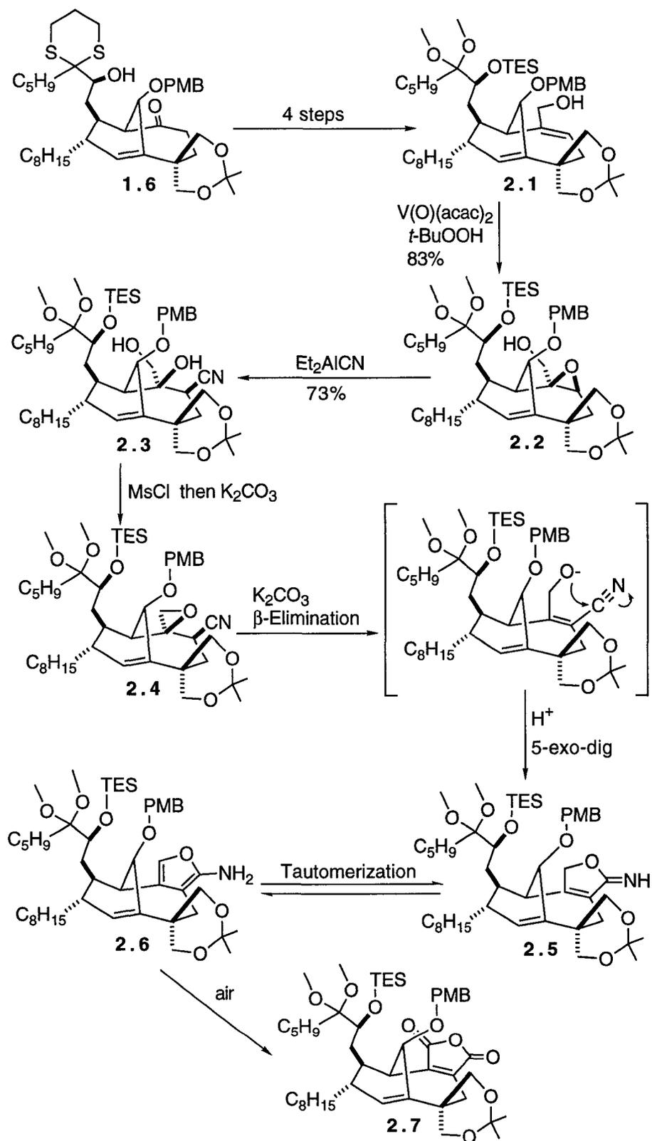
**Scheme 2.** Construction of maleic anhydride unit.
