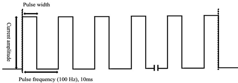
**Figure 1-2.** Schematic description of NMES parameters.
