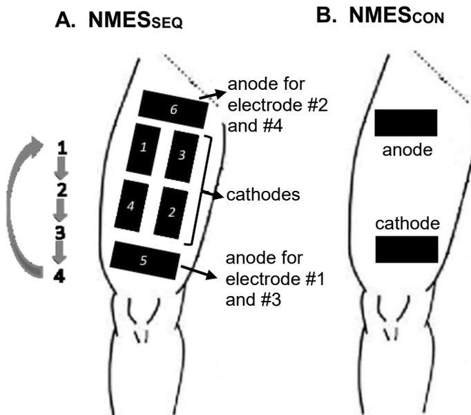
**Figure 2-1. Electrode placements.** Electrode placements for sequential (NMES<sub>SEQ</sub>; Panel A) and conventional NMES (NMES<sub>CON</sub>; Panel B). For NMES<sub>SEQ</sub>, pulses were rotated between cathodes at a net frequency of 40 Hz, resulting in a frequency at each cathode of 10 Hz. For NMES<sub>CON</sub>, the cathode was “fixed” and stimulus pulses were delivered at 40 Hz.
