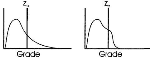
Figure 3.5: Distributions of uncertainty in grade for two blocks of material are shown. Note the long tail on the distribution on the left. If a probability of grade greater than the cutoff grade threshold were used for classification then both blocks would have the same probability of being classified as waste, but note that the distribution on the left has a higher probability of being ore.
