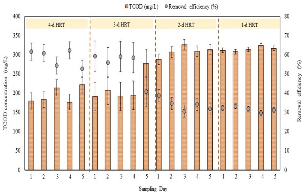
Figure 4.2: TCOD removal by MEC at different HRTs
