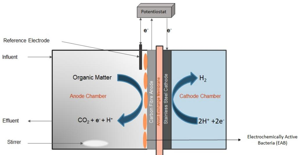
Figure 3.2: Schematic of Microbial Electrolysis Cell
