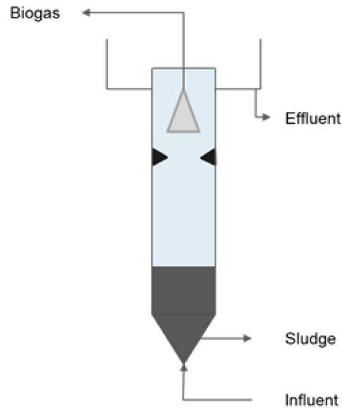
Figure 2.5: Upflow Anaerobic Sludge Blanket (UASB)
