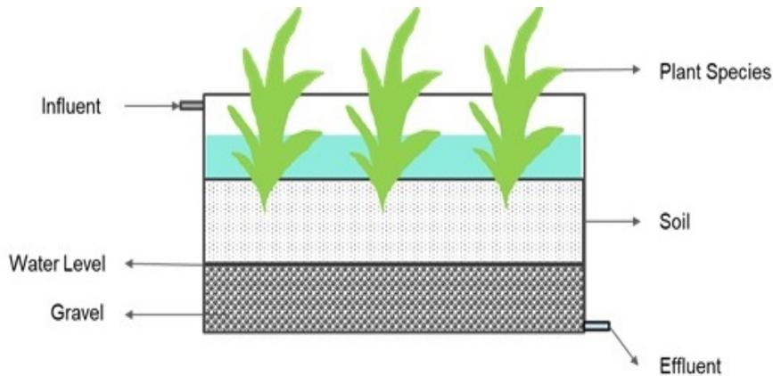
Figure 2.2: Constructed Wetland
