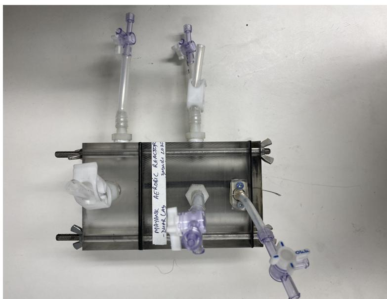
Figure A.5: GAC Biofilter Reactor
