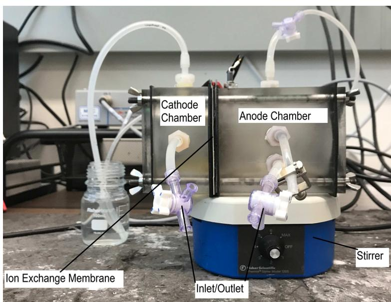
Figure A.4: MEC Reactor
