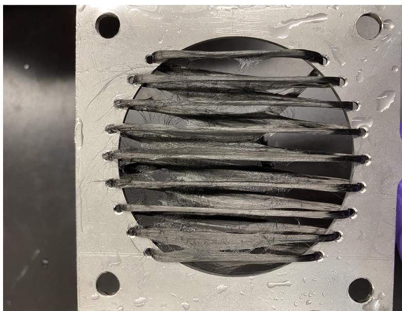
Figure A.3: Carbon Fiber Anode
