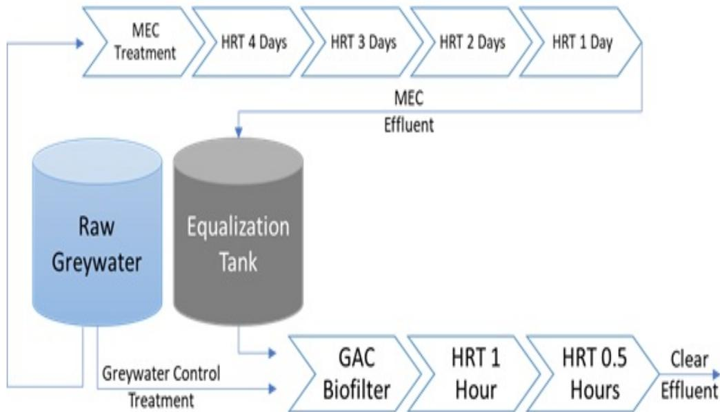
Figure 3.1: Schematic of the Treatment Process
