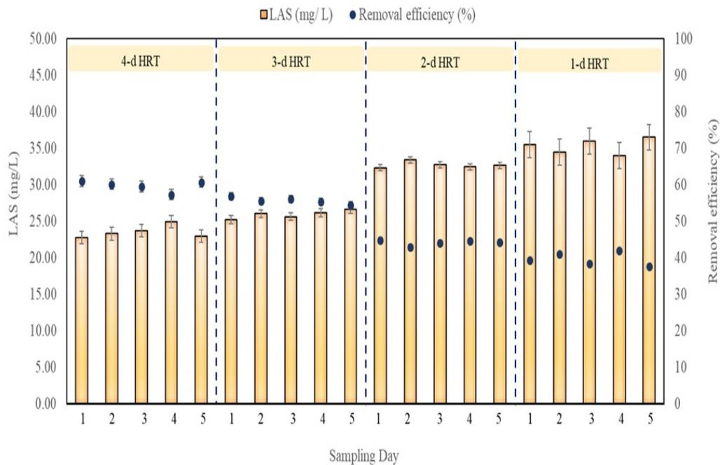
Figure 4.3: Removal and concentration of surfactants by MEC at different HRT
