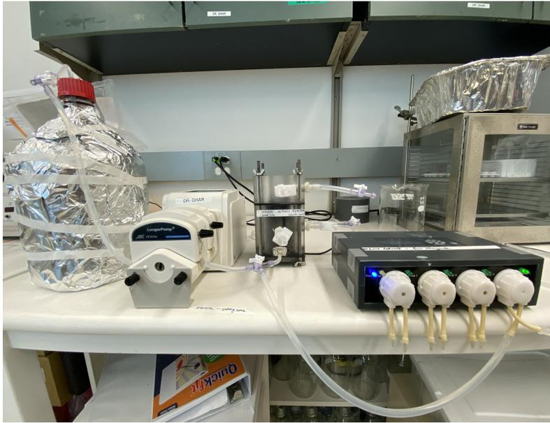
Figure A.1: Image of GAC-Biofilter Setup
