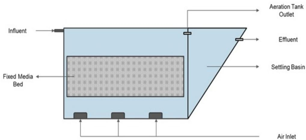
Figure 2.4: Integrated Fixedfilm Activated Sludge (IFAS)
