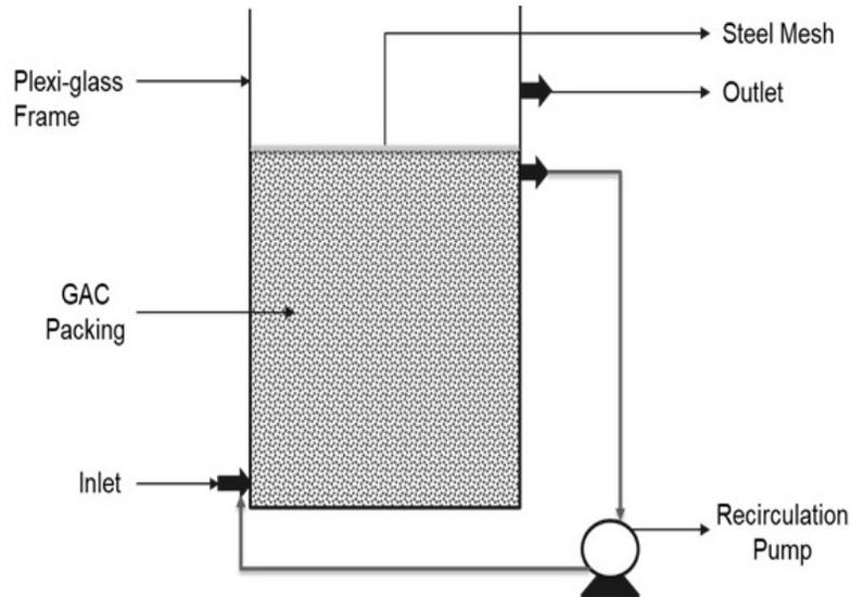
Figure 3.4: GAC-Biofilter Reactor
