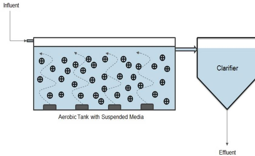
Figure 2.3: Moving Bed Biofilm Reactor (MBBR)
