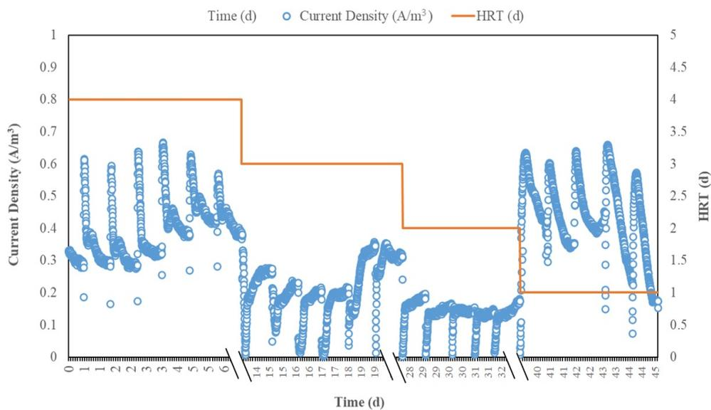
Figure 4.1: Volumetric Current Density in MEC at Different HRTs
