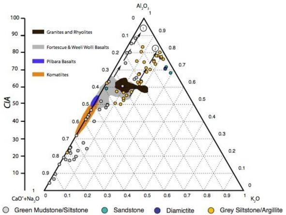
**Figure 2.12.** CIA plot for TCDP1 detrital sediments. Kungaara Formation shales appear to be weathered from a granite or rhyolite source, whereas shales within the Boolgeeda Iron Formation appear to represent an ultramafic to mafic source. Potassium enrichment can result from conversion of Al-rich clays to those more potassic in composition, such as illite or muscovite (Nesbitt and Young, 1989). Arrows 1 and 2 indicate weathering pathways of mafic and felsic rocks, respectively.
