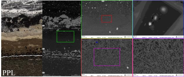
**Figure 4.6.** Location of nano-scale (~50-100 nm) spherical Fe-oxides. These features are found at the boundary of the dark mat layer and light mat layer. The coloured boxes outline the location of each blown up image.
