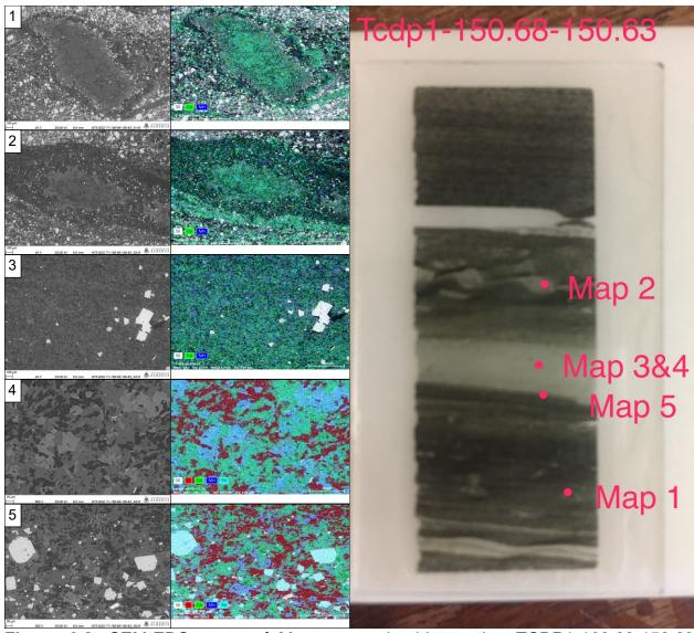
**Figure 3.8.** SEM-EDS maps of Mn textures in thin section TCDP1-160.68-150.63 corresponding to enrichment B1.
