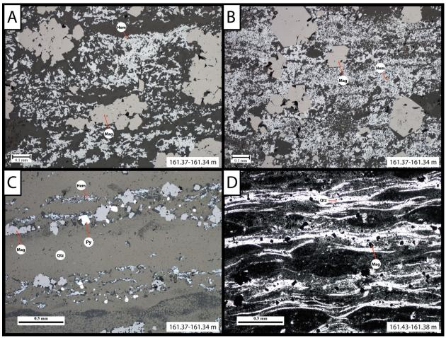
**Figure 2.4.** Typical textural associations of hematite and magnetite. A-B: Varying appearance of magnetite and hematite grains within closely spaced bands (<3 cm apart) under reflected light; hematite grains in B are smaller, less bladed, and more abundant than grains in A; magnetite grains in B are larger and more euhedral than in A. C: Microbanding similar to Trendall's (1973) type A under reflected light. D: Microbanding similar to Trendall's (1973) type B under transmitted light.
