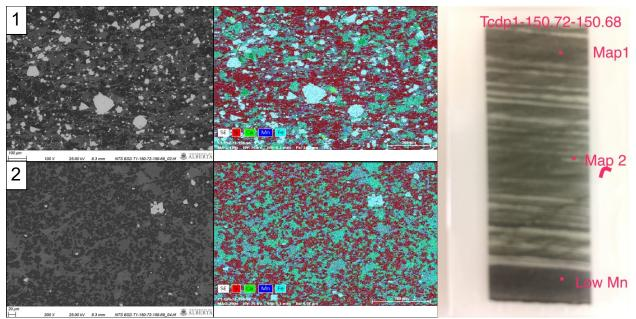
**Figure 3.9.** SEM-EDS maps of Mn textures in thin section TCDP1-150.72-150.68 corresponding to enrichment B1.
