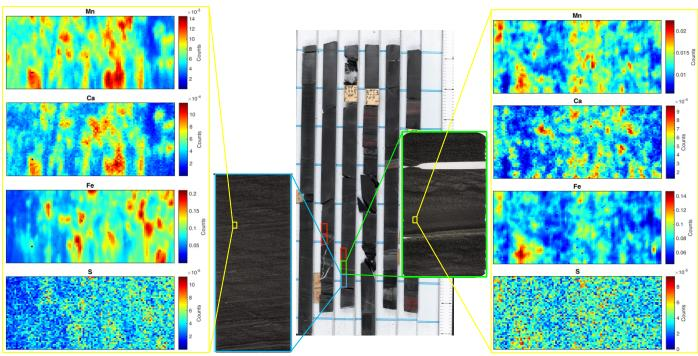
**Figure 3.10.**  $\mu$ XRF mapping for samples T1-150.73-150.68 and T1-150.68-150.63 (B1). The blue and green boxes highlight the location of thin sections T1-150.73-150.68 and T1-150.68-150.63, respectively. The location of XRF maps is highlighted in yellow. Maps are 1mm x 2mm in size. Mn is concentrated in carbonate grains that concentrate in thin layer, banded on the mm-scale.
