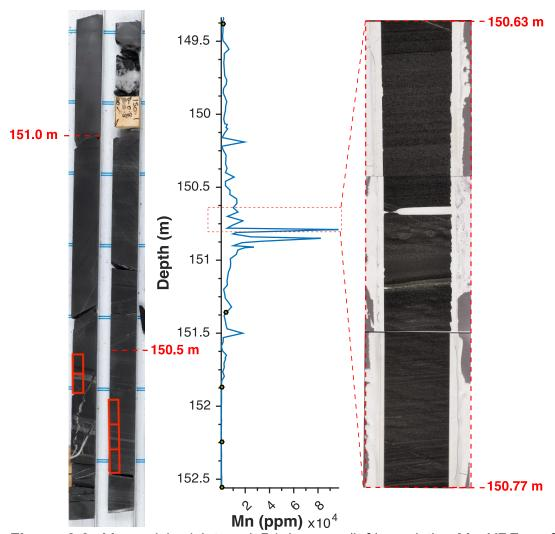
**Figure 3.6.** Mn enriched interval B1 in core (left), and the Mn XRF profile (center) spanning this section. Magnified images of thin sections (right) have been included to show carbonate textures within the interval. Note the spherical features separating Mn enriched beds below from Mn depleted beds above. Red boxes on the core photos indicate where thin sections were taken.
