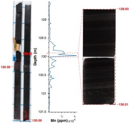
**Figure 3.12.** Mn enriched interval B2 in core (left), and the Mn XRF profile (center) spanning this section. Magnified images of thin sections (right) have been included to show carbonate textures within the interval. Red boxes on the core photos indicate where thin sections were taken.
