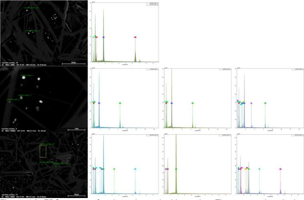
**Figure 4.9.** EDS spectra of various phases in thin section. The nano-scale spherical features in the mat layer are Fe-oxides. Surrounding matrix is silica. The bladed mineral is some form of Fe, K, Al, Mg clay (perhaps diagenetic product of mat degradation?). The spaces in between the clays are completely silicified. This mat may have been preserved by silicification as overlying BIF deposition took place.
