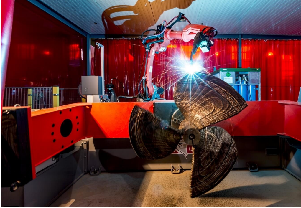
Figure 2.2 World's first ship propeller fabricated with WAAM in 2017 by RAMLAB
