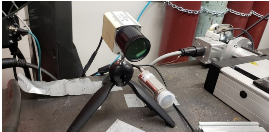
Figure 3.12 IR camera mounted on tripod perpendicular to direction of deposited wall
