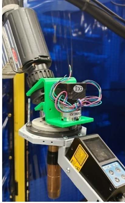
Figure 4.6 Profilometer attached behind and along the trajectory of the print path
