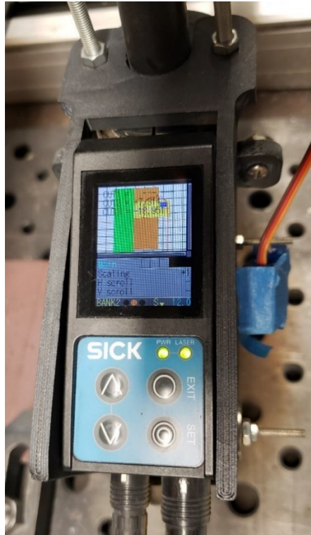
Figure 3.5 Top view of mounted profiler with graphical user interface displaying the profile of the bead on the substrate
