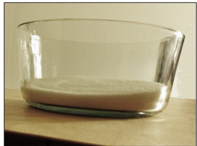
Figure 3. Granulated sugar measured out into a dish to make a solution for sorting chironomid larvae from a substrate sample by flotation (about 2 cups [475 ml]). An effective solution is obtained by adding about twice this volume of water, for a specific gravity of 1.12.
