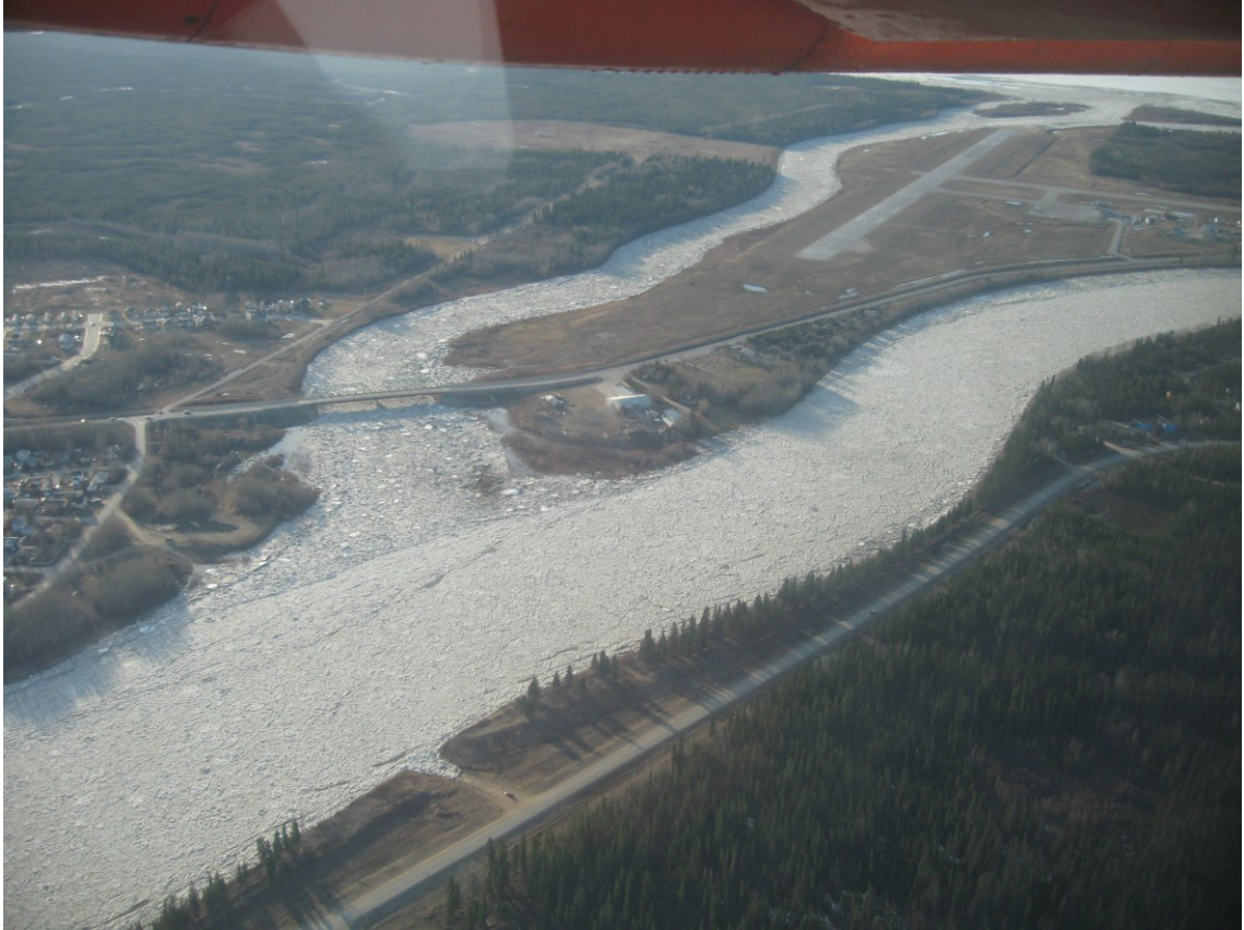
Figure 1.3. An ice jam in the multi-channel Hay River delta. The flow direction is from bottom left to top right.
