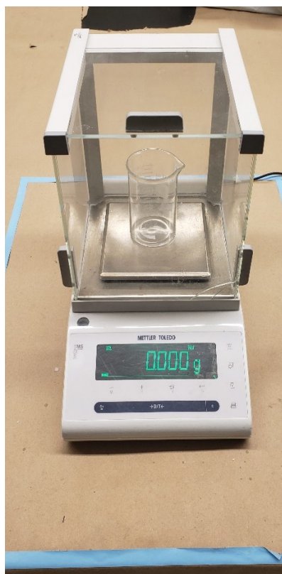
b) Scale used to weigh EBC collection on masks
