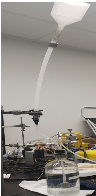
a) EBC exposure bubbler set-up
