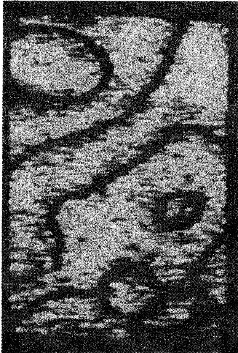
Figure-2.14: 25 \mu m sensitivity ESPI contour fringes defining the difference between a section of master turbine blade and inspection blade. The position of these fringes had been identified and enhanced by computer analysis 1 [Taken from Ref. 1 with kind permission of Dr. R. Jones, p.292].
