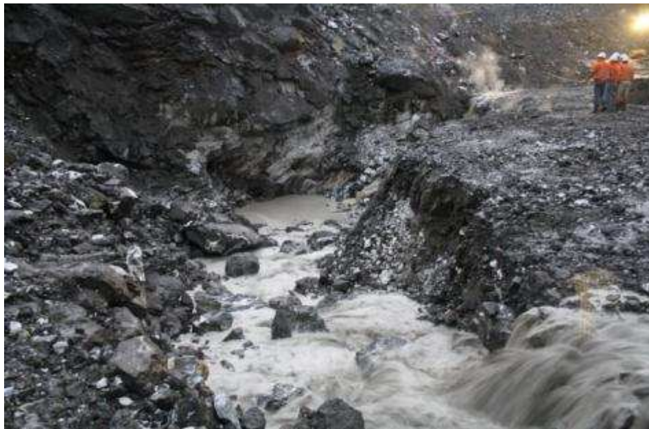
Figure 35: Cavities observed in the Lienetz Pit (Lihir Gold Ltd)
