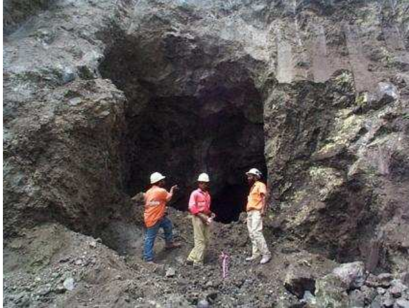
Figure 34: Cavities observed in the Lienetz Pit (Lihir Gold Ltd)
