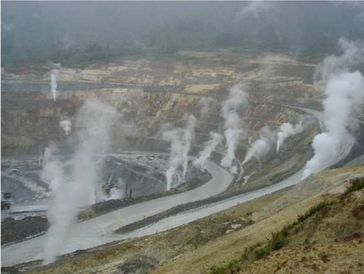
Figure 42: Steam relief wells in Liepitz Pit
