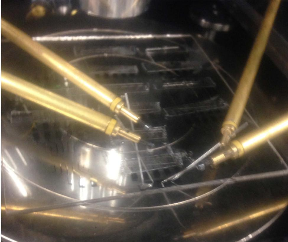
Figure 4.4. Flow cell substrate, featuring nine locations for flow cells. Device is rotated 180° from the design in Figure 4.3. Four probe tips in a probe station on a Pt test contact pad are shown. The probe tips are connected to a Keithley 4200 semiconductor characterization system. Square glass substrate shown is 10 cm x 10 cm.
