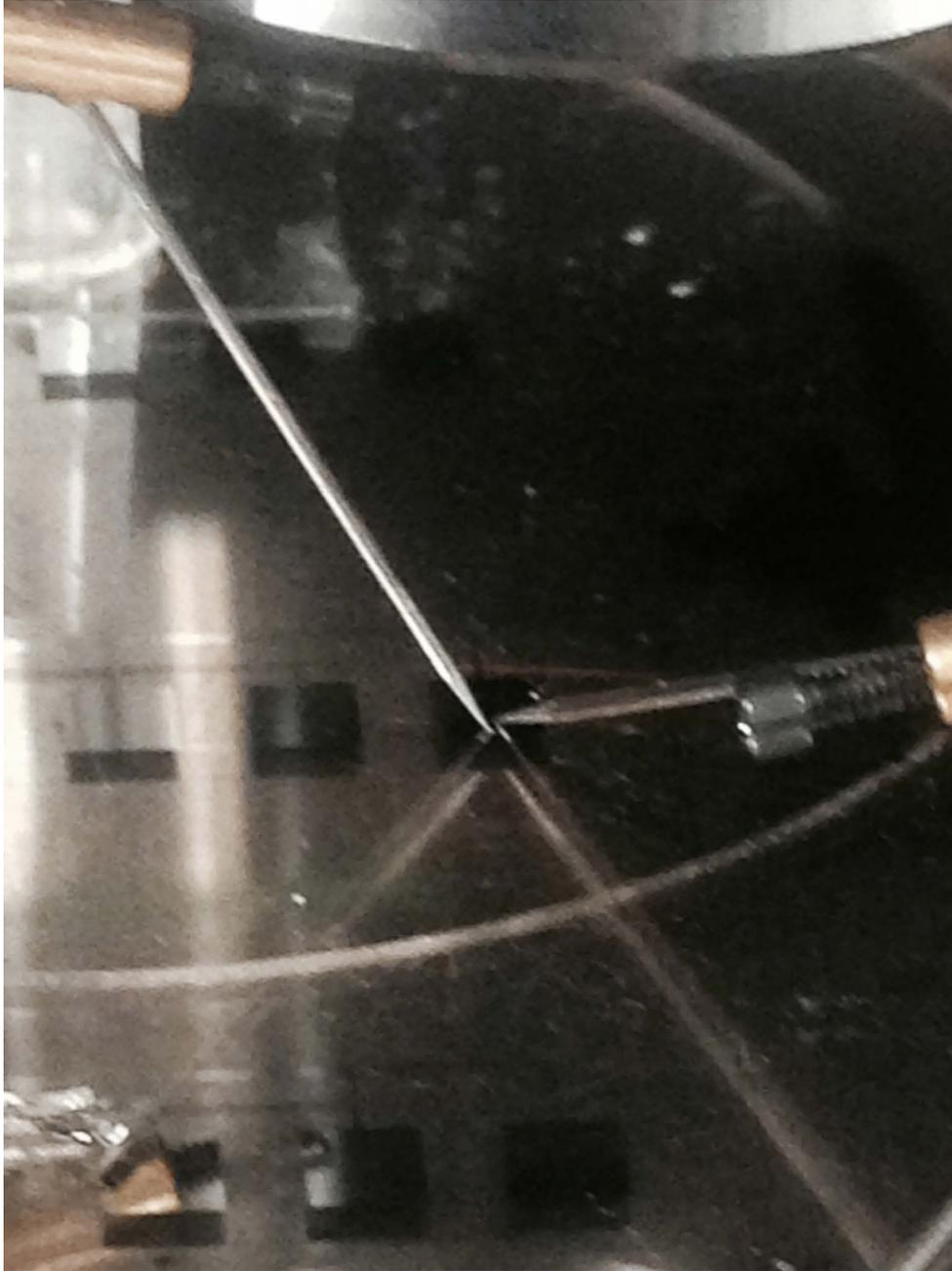
Figure 4.39. Probe tips making resistance measurement on a metal contact pad.
