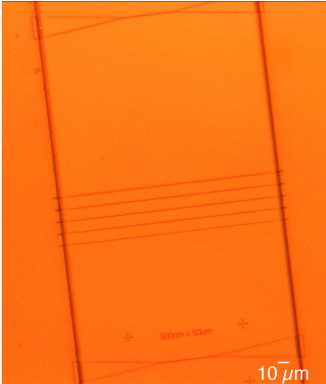
Figure 4.49. 20x optical image of D3 after creation of nanochannels. The bottom and top channels are 500nm wide, and the middle nanochannels are designed to be 200, 300, 400, 600, 800, and 1000 nm, starting from the bottom (the 200nm channel is barely visible).
