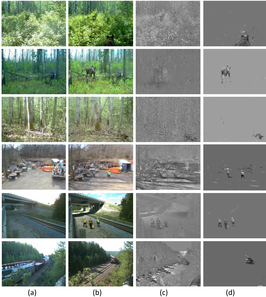
Figure 5.12: (Columns (a) and (b): two selected images of each sequence, (c) and (d): illumination changes captured in \mathcal{C} , and detected objects of images in (b), respectively
