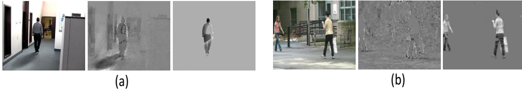
Figure 5.7: Columns from left to right show sample image, illumination changes, and detected moving objects for (a) cubicle and (b) backdoor sequences
