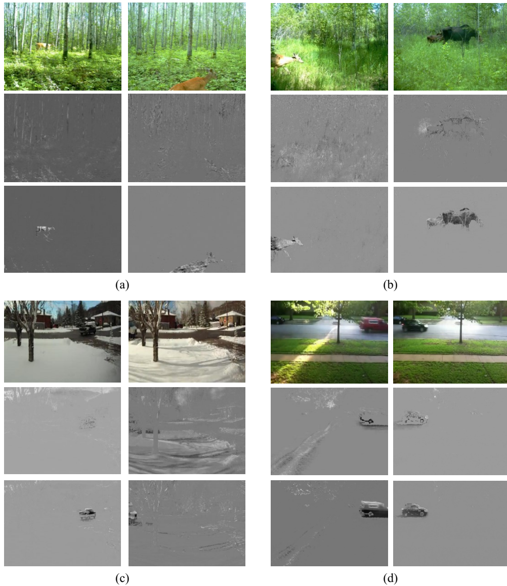
Figure 4.14: First row: two sample images with different illumination for each sequence. Second row: sparse outliers C . Third row: detected objects S .
