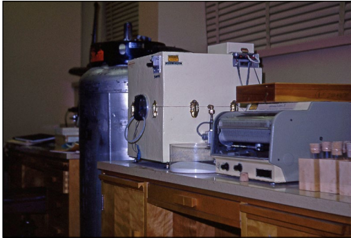
Fig. 3. An apparatus built in 1969 to measure insect supercooling points, and operated by liquid nitrogen.
