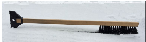
Fig. 4. A simple automobile snow-brush, showing the toothed side of the ice-scraper blade (total length 64 cm).
