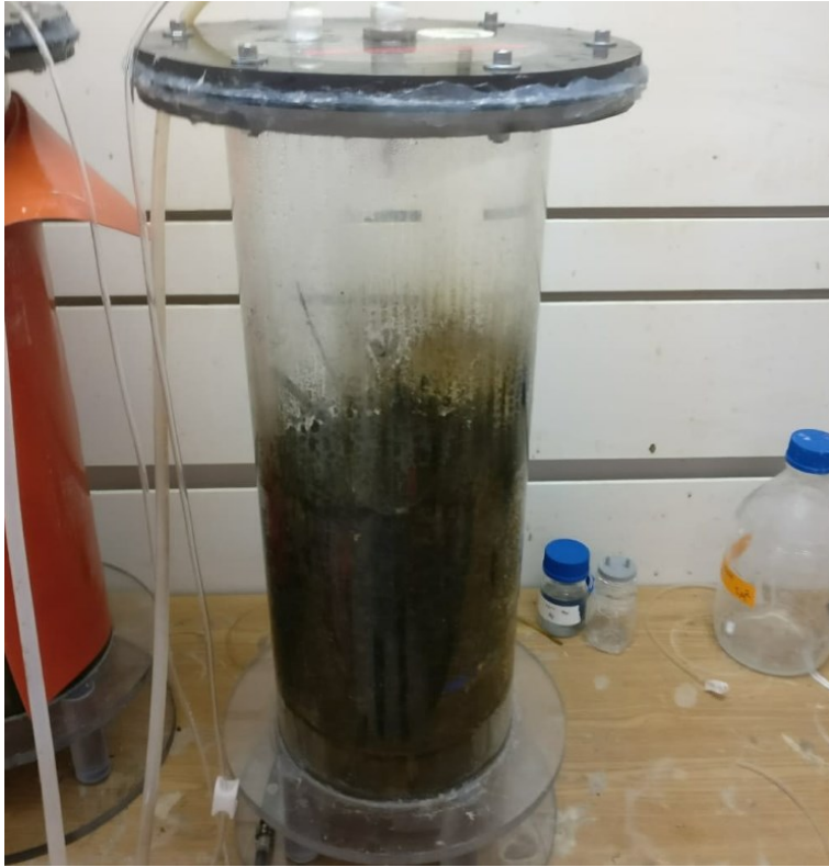
Fig. A.5 Photo of solid digester with digestate
