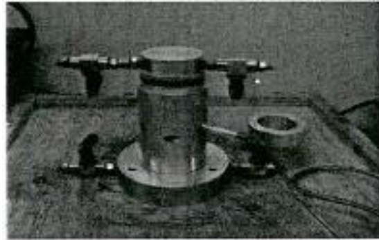
Figure 3.15: Place the top cap on
