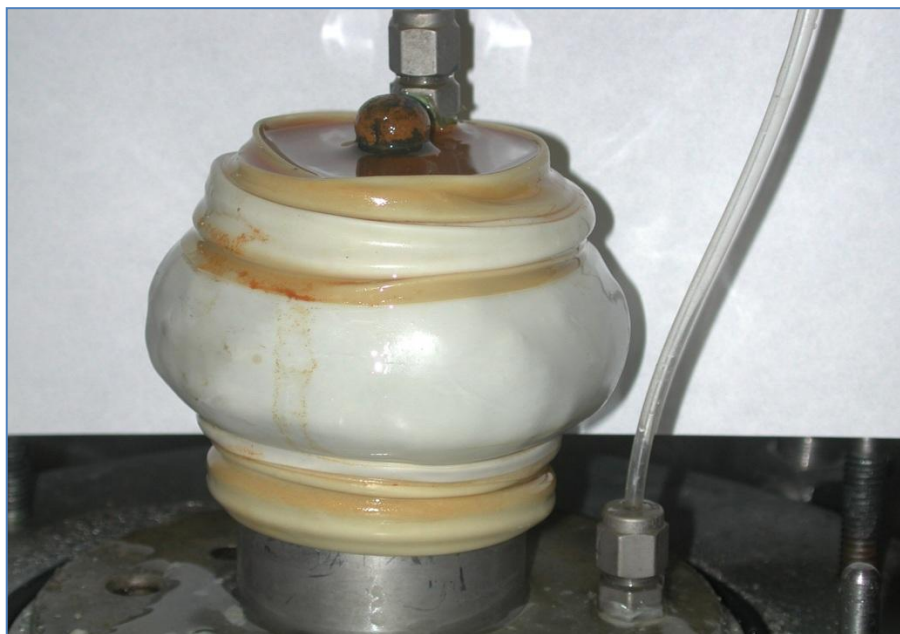
Figure 4.19: Effect of end platens on specimen at the end of shearing.
