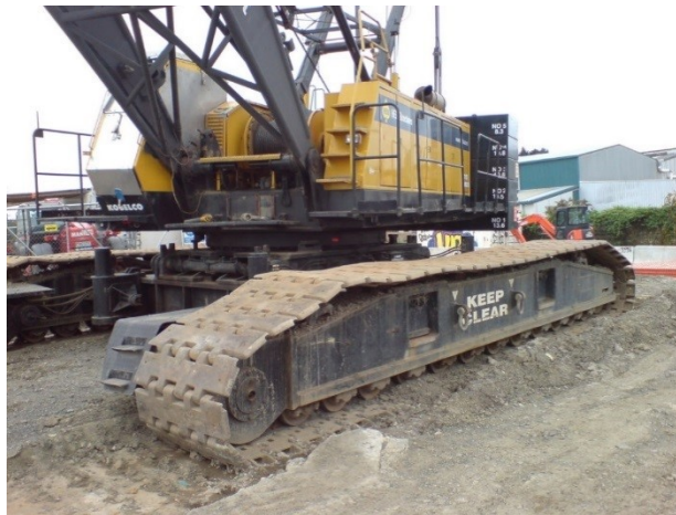
Fig. 3-12: Crawler crane track
