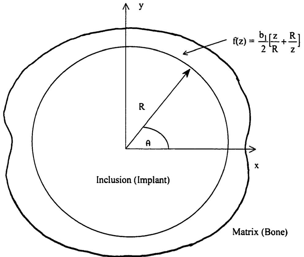
**Figure 6 - 1.** Schematic Representation of the Inhomogeneous Non-Slip Interface having Circumferential Number  $s = 1$
