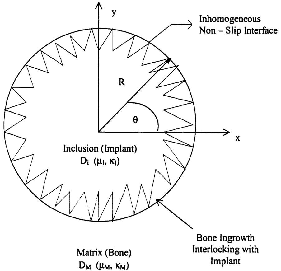
**Figure 5-1.** A Homogeneous Circular Inclusion with Circumferentially Inhomogeneous Non – Slip Interface
