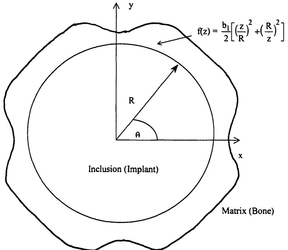
Figure 6 - 9. Schematic Representation of the Inhomogeneous Non - Slip Interface having Circumferential Number  $s = 2$
