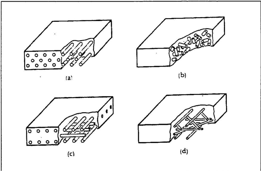
**Figure 1-2.** Several Orientations of Fiber-Reinforced Composites: (a) Continuous Unidirectional Fibers, (b) Randomly Oriented Short Discontinuous Fibers, (c) Orthogonal Fibers, and (d) Multiple-Ply Fibers (From Donald R. Askeland, *The Science and Engineering of Materials*, Second S.I. Edition, Chapman & Hall 1990)
