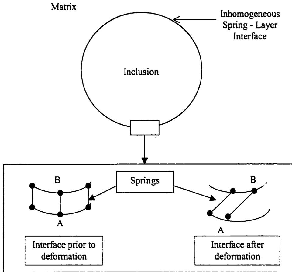
**Figure 3-1.** Schematic Representation of Inhomogeneous Spring - Layer Interface before and after Deformation
