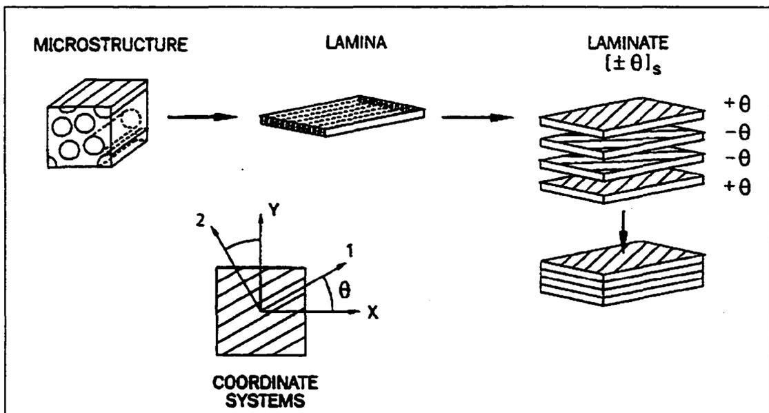
**Figure 1-4.** Schematic Representation of Fiber-Reinforced Laminate Composite (From John Wolodko, *Biaxial Fatigue and Leakage Characteristics of Fiber Reinforced Composite Tubes* Ph. D. Thesis, University of Alberta, 1999)
