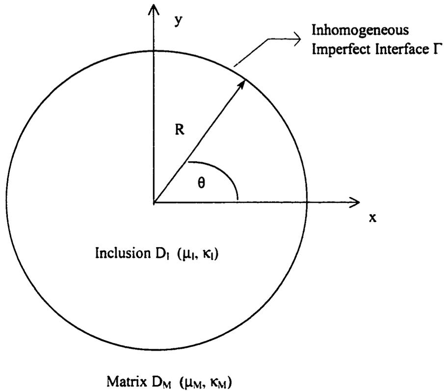
**Figure 2-1.** A Homogeneous Circular Inclusion with Circumferentially Inhomogeneous Imperfect Interface Embedded in an Infinite Elastic Matrix in Plane Elasticity
