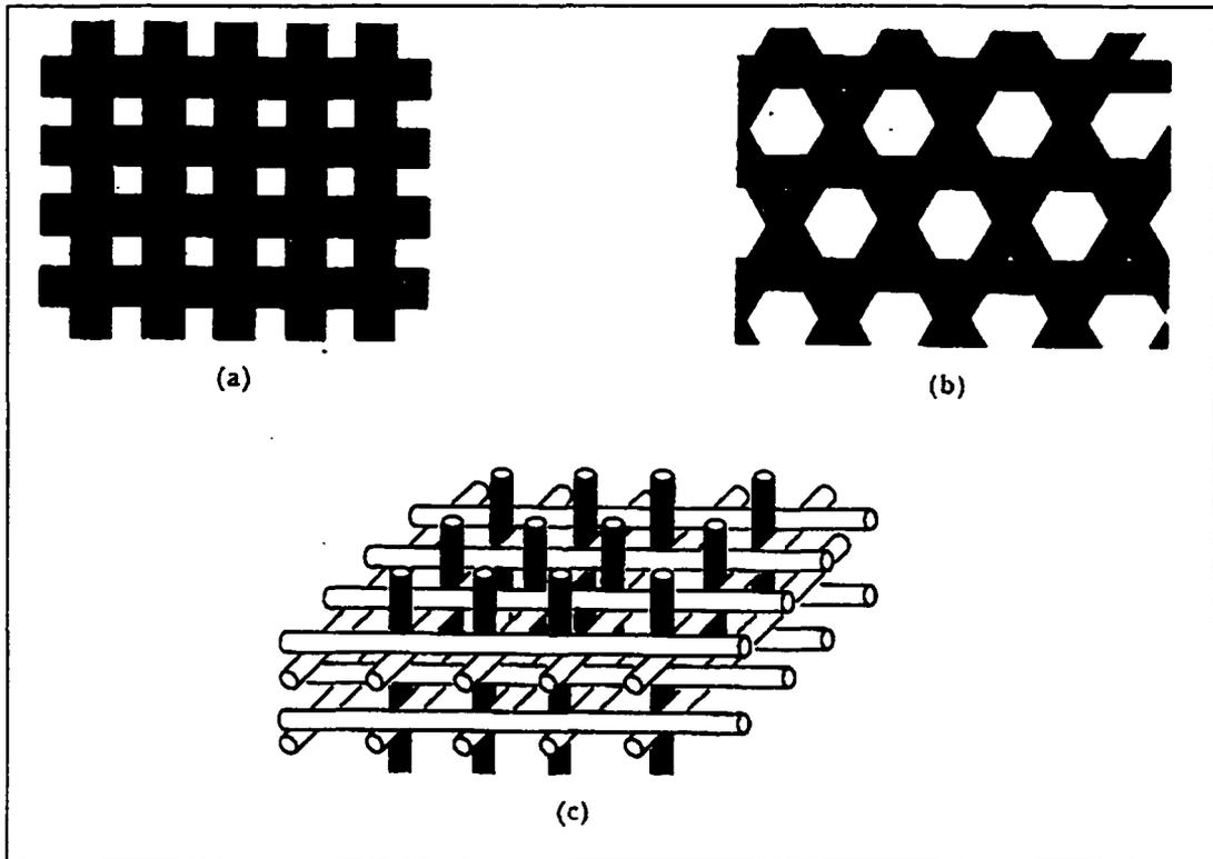
**Figure 1-3.** Several Weave Patterns for Fibers: (a) Biaxial Weave, (b) Triaxial Weave, and (c) Three-Dimensional Weave (From Donald R. Askeland, *The Science and Engineering of Materials*, Second S.I. Edition, Chapman & Hall, 1990)
