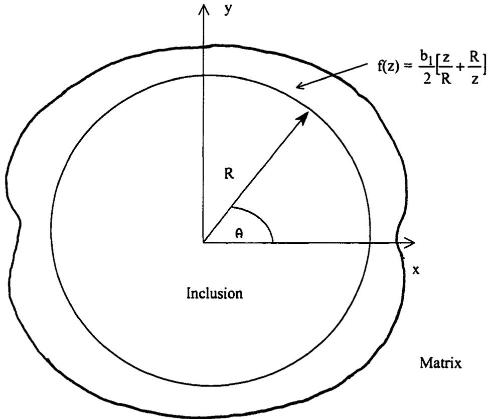
**Figure 4 - 1.** Schematic Representation of the Inhomogeneous Spring – Layer Interface having Circumferential Number  $s = 1$
