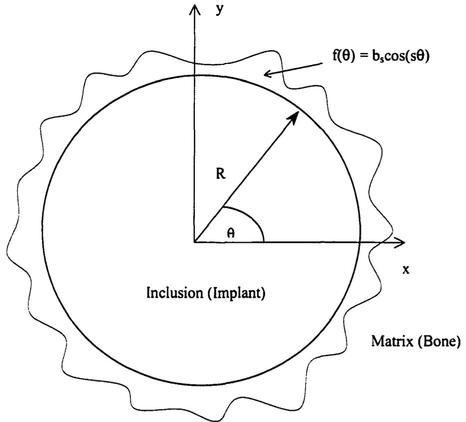
**Figure 5-2.** Schematic Representation of the Inhomogeneous Non – Slipping Interface
