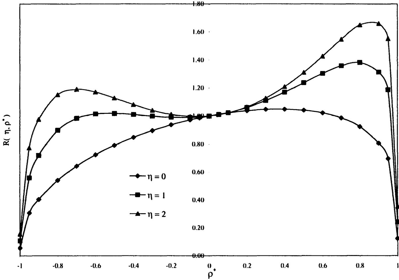
**Figure 4-6.** The Effect of the Circumferential Inhomogeneity on the Average Deviatoric and Shear Stress inside the Circular Inclusion having Circumferential Number  $s = 2$  and Loading in x-direction
