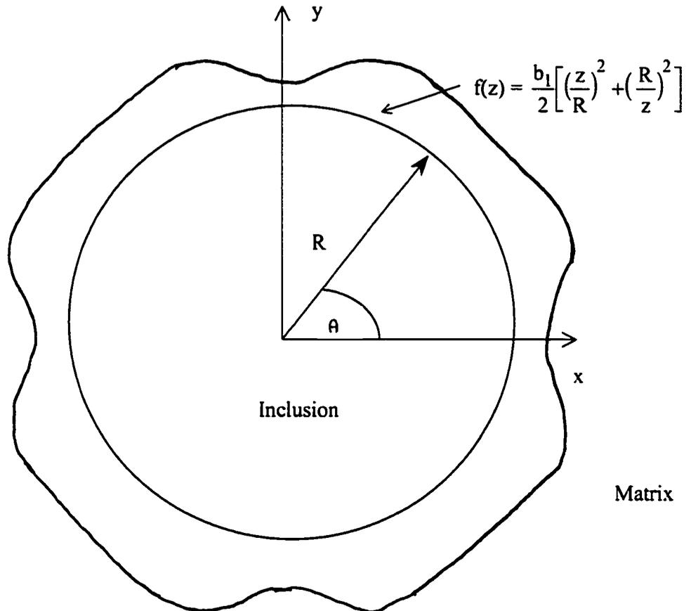
**Figure 4 - 4.** Schematic Representation of the Inhomogeneous Spring - Layer Interface having Circumferential Number  $s = 2$
