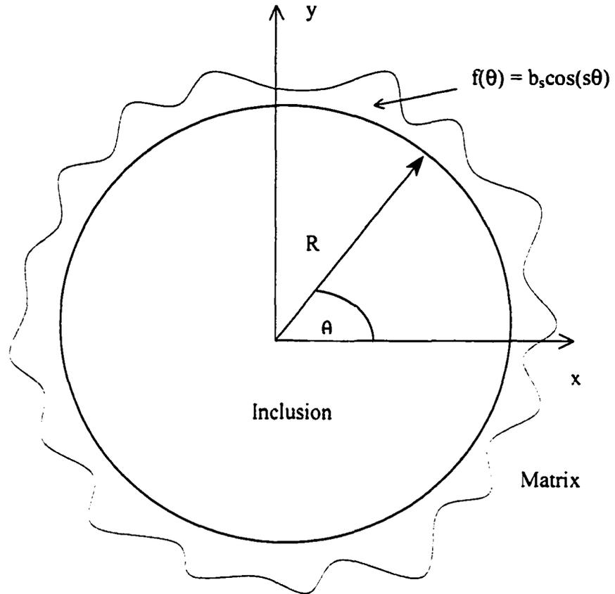
**Figure 3-2.** Schematic Representation of the Inhomogeneous Spring – Layer Interface
