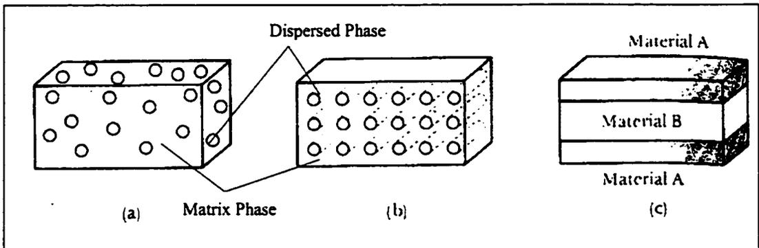
**Figure 1-1.** Three Types of Composite Materials: (a) Particulate Composite, (b) Fiber-Reinforced Composite, and (c) Laminar Composite
