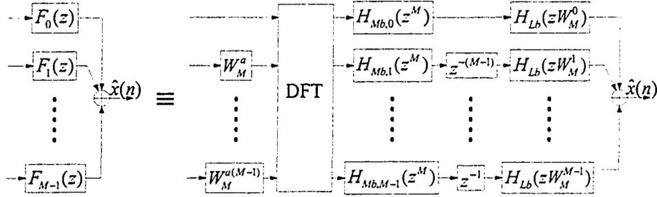
Figure 4.7: Realization of the synthesis filters  $F_k(z)$  in terms of the polyphase components of  $H_{Mb}(z)$  for a narrow-band FRM prototype digital filter  $P(z)$
