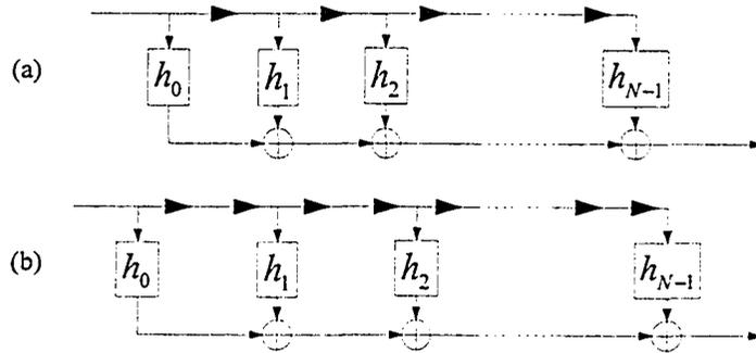
Figure 3.20: The realization of (a) a FIR digital filter, and (b) its modification for 2-fold interleaving
