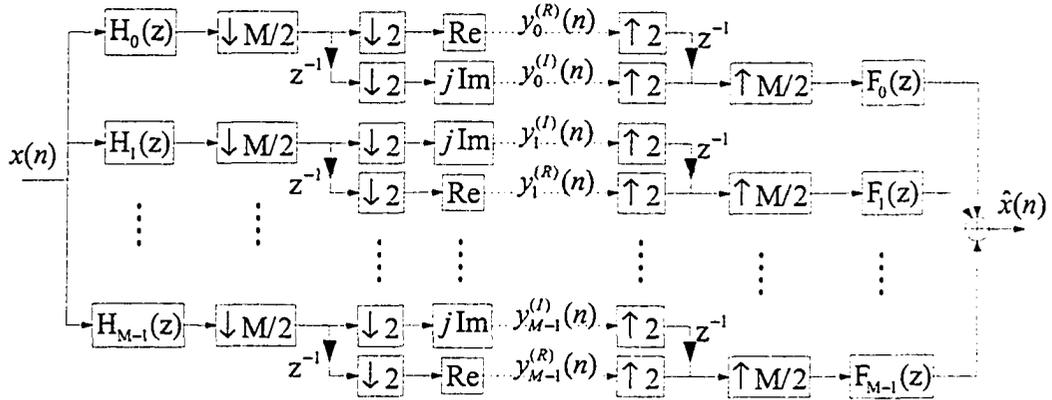
Figure 2.12: The Structure of a  $M$ -channel MDFT filterbank
