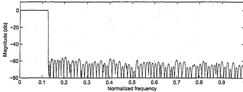
Figure 4.20: Magnitude-frequency response of the arbitrary bandwidth FRM prototype digital filter  $P(z)$  in Example 2
