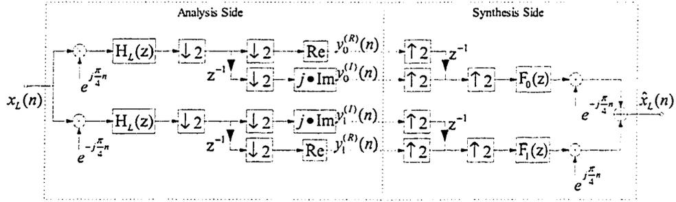
Figure 3.9: Detailed structure of the  $L$ -th subsystem
