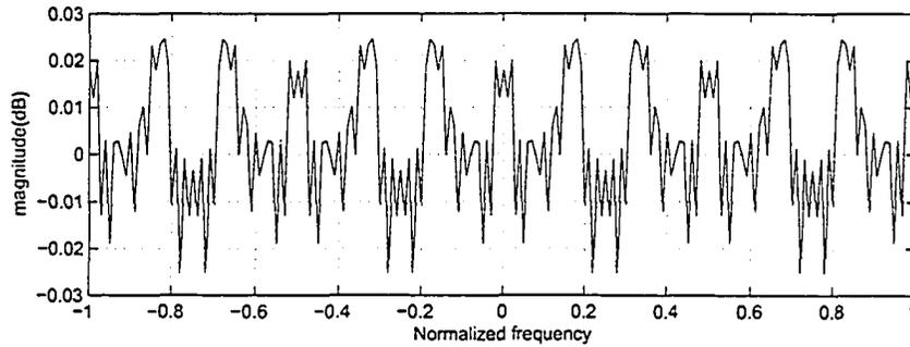
Figure 3.32: The overall distortion for the 6-stage filterbank
