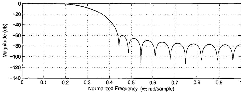
Figure 3.24: Magnitude-frequency response of the last-stage filters  $H_L(z)$  employing the windowing approach
