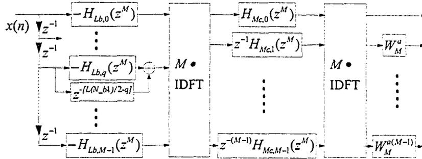
Figure 4.9: Realization of the second term in the right-hand side of Eqn. 4.25, based on an arbitrary-bandwidth FRM digital filter  $P(z)$
