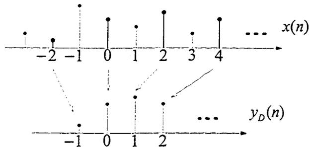
Figure 1.3: The decimation operation in time-domain (for  $M = 2$ )
