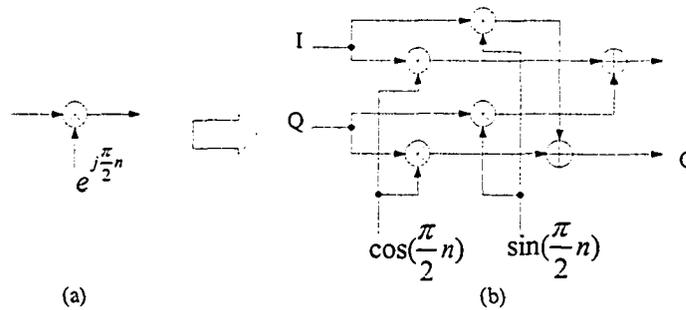
Figure 3.22: Real processing of complex signal sequences
