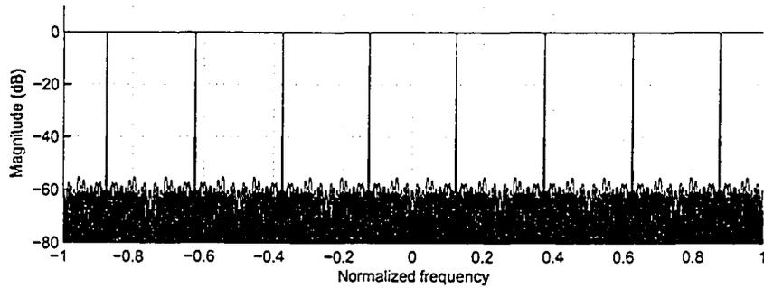
Figure 4.21: Magnitude-frequency response of the analysis filterbank in Example 2
