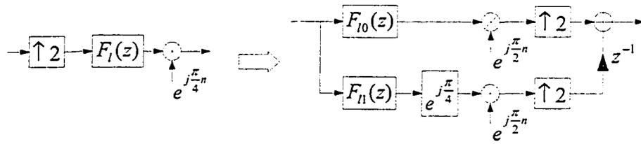
Figure 3.19: Equivalence for *Stage l'* reconstruction modules
