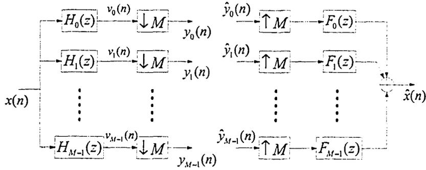
Figure 2.2: The  $M$ -channel maximally-decimated filterbank
