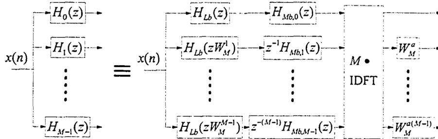
Figure 4.4: Realization of the analysis filters  $H_k(z)$  in terms of the polyphase components of  $H_{Mb}(z)$  for a narrow-band FRM prototype digital filter  $P(z)$
