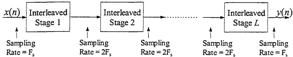
Figure 3.21: Realization of the interleaved tree-structured filterbank
