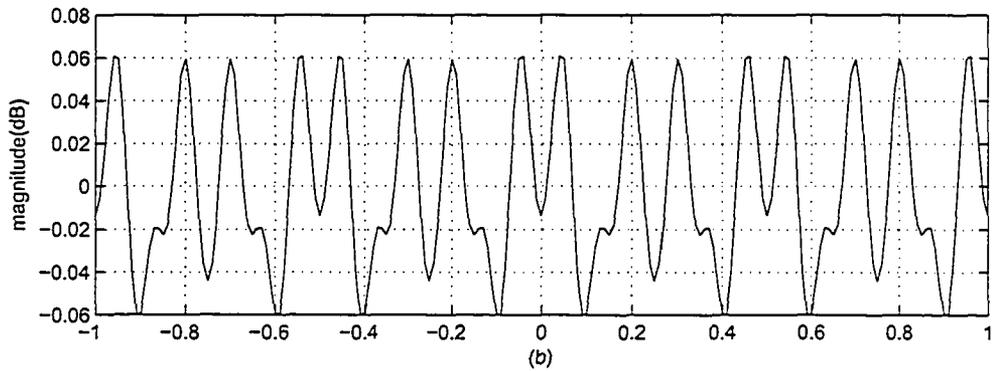
Figure 3.27: (a) The overall distortion of the 3-Stage filterbank using windowing technique with low passband ripple intermediate stage filters  $H_l(z)$
