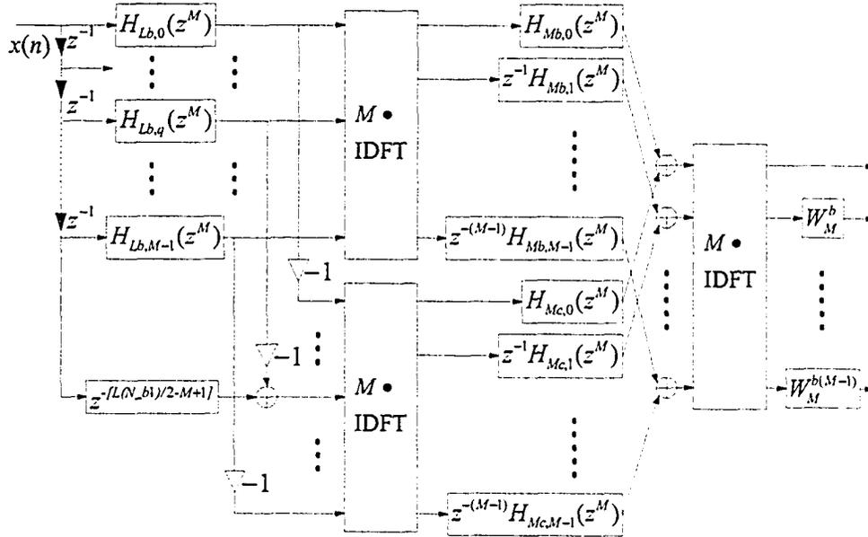
Figure 4.10: Realization of the analysis filters  $H_k(z)$  in terms of the polyphase components of  $H_{Lb}(z)$  and  $H_{Mb}(z)$  for an arbitrary-bandwidth FRM prototype digital filter  $P(z)$
