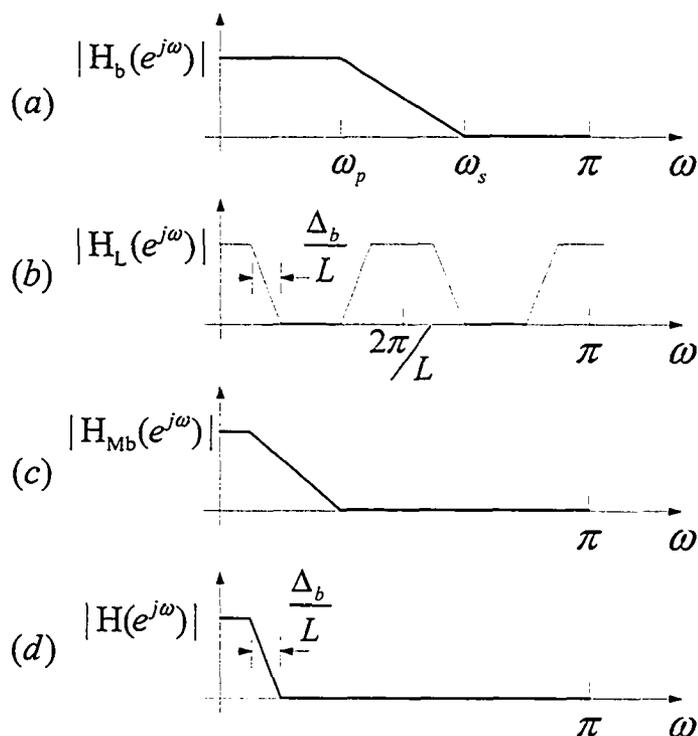
Figure 4.1: Magnitude-frequency responses for obtaining a narrow-band FRM digital filter  $H(z)$
