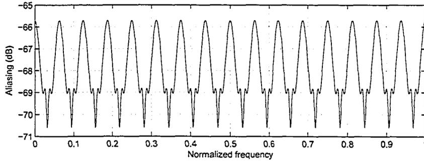
Figure 4.17: Aliasing function  $A(z)$  for the MDFT filterbank in Example 1
