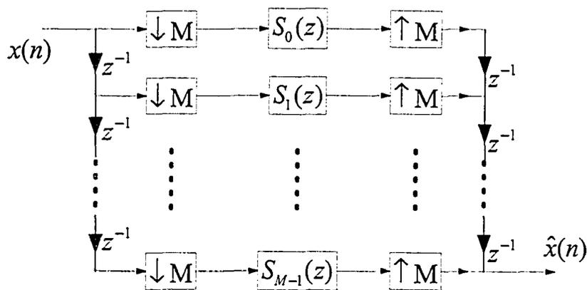
Figure 2.10: A general  $M$ -channel multirate DSP system
