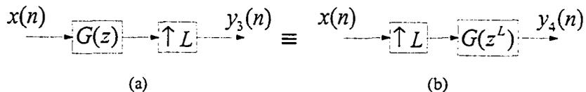
Figure 1.8: Identity involving interpolators
