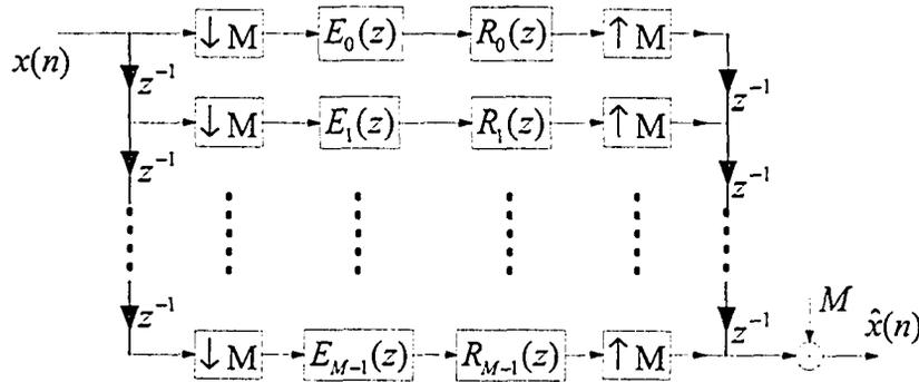
Figure 2.11: The equivalent representation of a maximally-decimated  $M$ -channel DFT analysis and synthesis filterbanks
