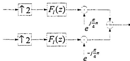
Figure 3.4: Intermediate *Stage  $l'$*  modules for synthesis filterbanks
