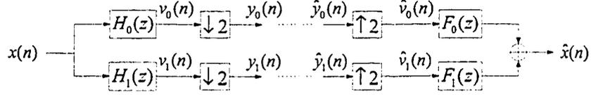
Figure 2.1: The structure of the basic QMF filterbank
