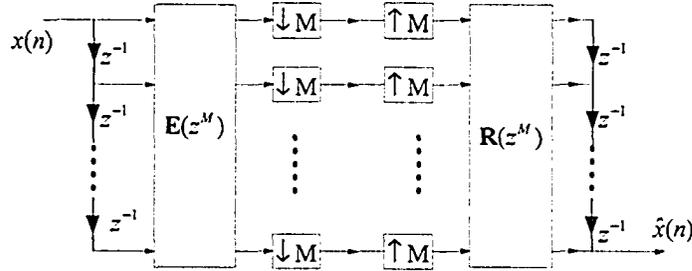
Figure 2.5: Equivalent polyphase representation of an  $M$ -channel maximally-decimated filterbank
