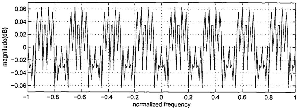
Figure 3.28: The overall distortion of 6-stage filterbank (window approach)
