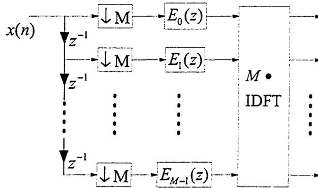
Figure 2.8: Simplified structure of a maximally-decimated  $M$ -channel DFT analysis filterbank
