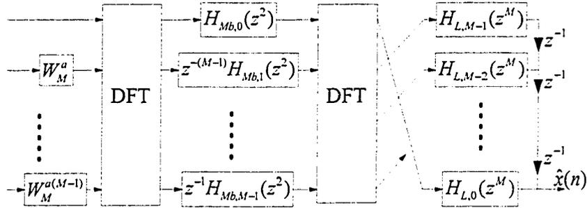
Figure 4.8: Realization of the synthesis filters in terms of the polyphase components of  $H_{Lb}(z)$  and  $H_{Mb}(z)$  for a narrow-band FRM prototype digital filter  $P(z)$
