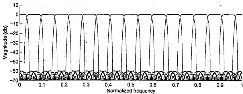
Figure 4.15: Magnitude-frequency responses associated with the proposed  $M$ -channel MDFT filterbank in Example 1
