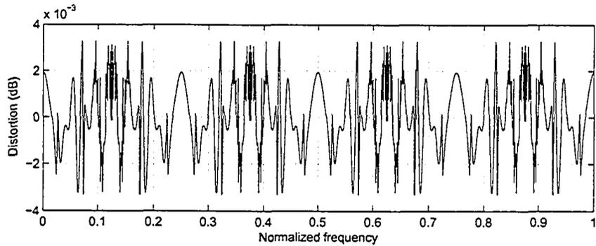
Figure 4.22: Deviation from a unity magnitude-frequency response for the MDFT filterbank in Example 2
