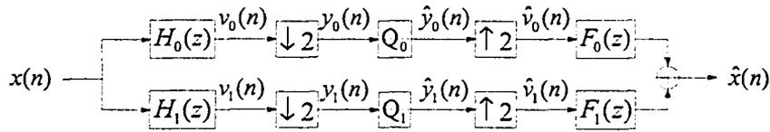
Figure 1.11: The structure of a basic QMF filterbank for SBC
