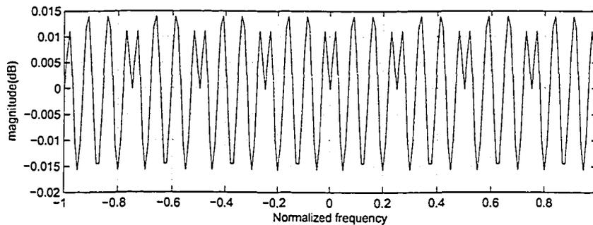
Figure 3.31: The overall distortions for the 3-stage filterbank
