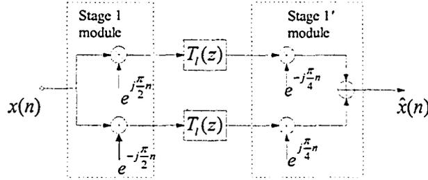
Figure 3.17: Alternative  $L$ -stage filterbank (including analysis and synthesis sides)
