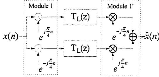
Figure 3.13: Alternative 2-stage filterbank (including analysis and synthesis sides)
