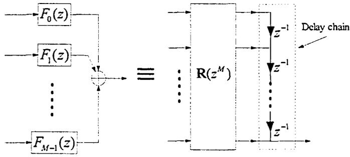
Figure 2.4: Type 2 polyphase representation of a  $M$ -channel synthesis bank
