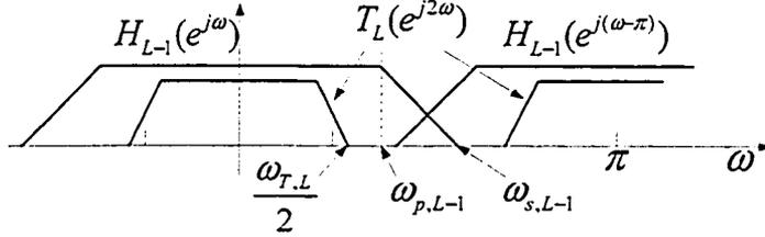
Figure 3.15: Relationships between the frequency characteristics of  $H_{L-1}$  and  $H_L$
