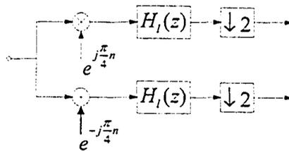
Figure 3.3: Intermediate *Stage  $l$*  modules for analysis filterbanks
