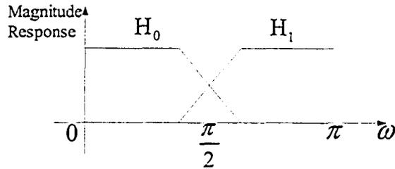
Figure 1.12: The magnitude frequency-response characteristics of analysis filters
