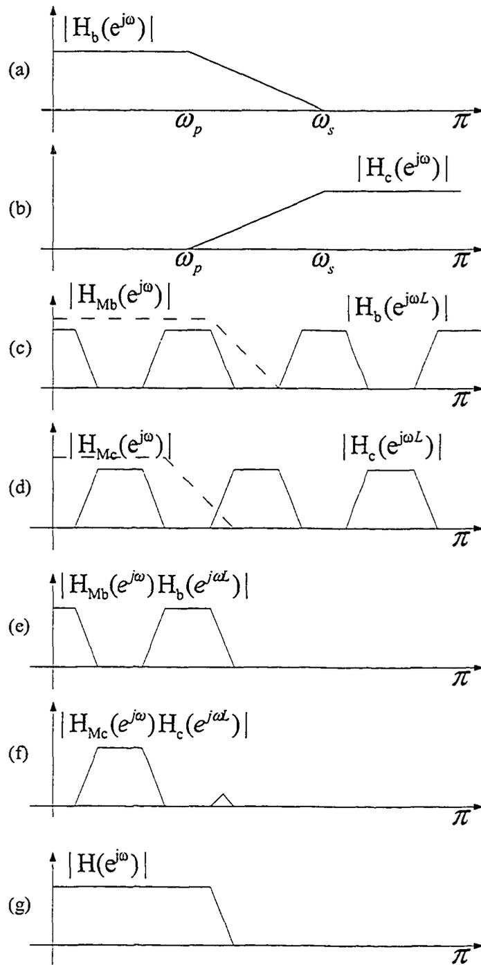
Figure 4.2: Magnitude-frequency responses for obtaining an arbitrary-bandwidth FRM digital filter  $H(z)$
