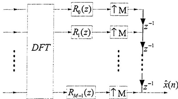
Figure 2.9: The structure of a maximally-decimated  $M$ -channel DFT synthesis filterbank
