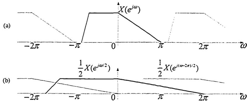
Figure 1.4: The decimation operation in frequency-domain (for  $M = 2$ )
