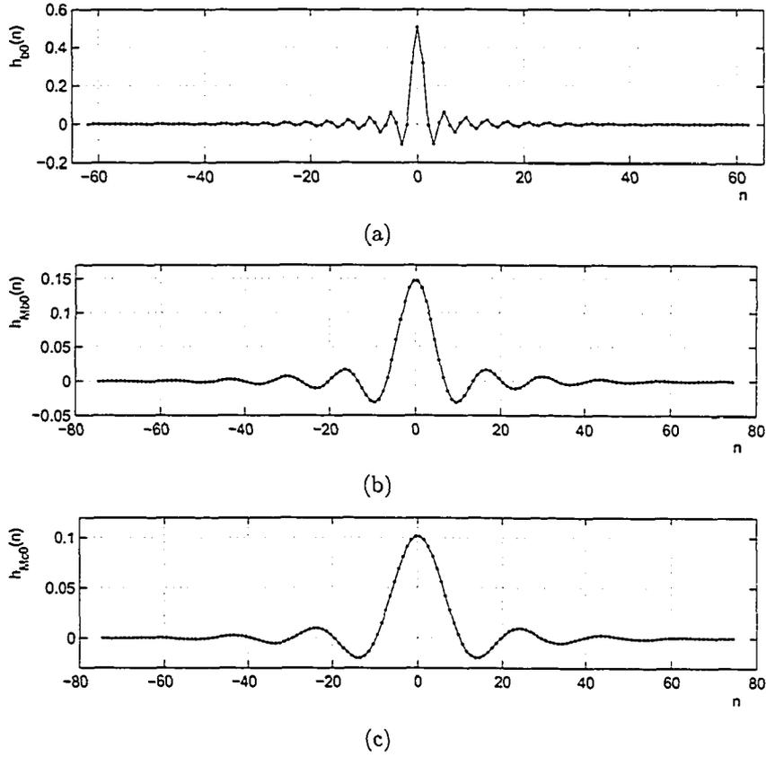
Figure 4.18: Multiplier coefficient values for (a) filter  $H_{b0}(z)$ , (b) masking filter  $H_{Mb0}(z)$ , and (c) masking filter  $H_{Mc0}(z)$
