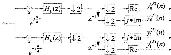
Figure 3.5: Internal structure of *Stage L* modules
