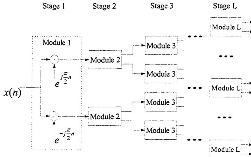
Figure 3.1: Multistage tree-structured analysis filterbank
