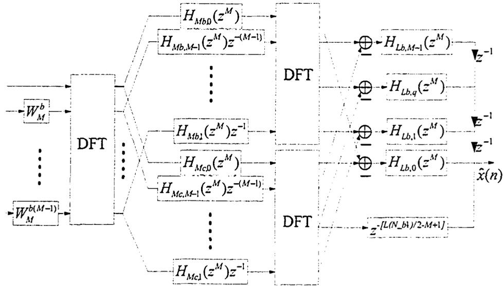
Figure 4.11: Realization of the synthesis filters  $F_k(z)$  in terms of the polyphase components of  $H_{Lb}(z)$  and  $H_{Mb}(z)$  for an arbitrary-bandwidth FRM prototype digital filter  $P(z)$
