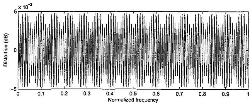
Figure 4.16: Distortion from a unity magnitude-frequency response for the MDFT filterbank in Example 1
