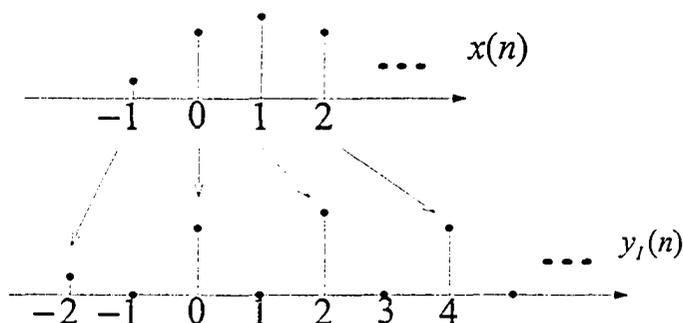
Figure 1.5: The interpolation operation in time-domain (for  $L = 2$ )
