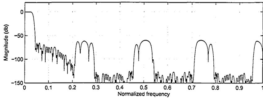
Figure 4.14: Magnitude-frequency response of the FRM prototype digital filter  $P(z)$  in Example 1
