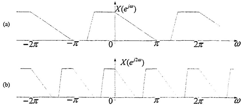
Figure 1.6: The interpolation operation in frequency-domain (for  $L = 2$ )
