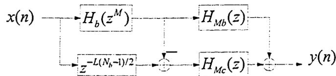
Figure 4.3: Realization of the arbitrary-bandwidth FRM digital filter  $H(z)$
