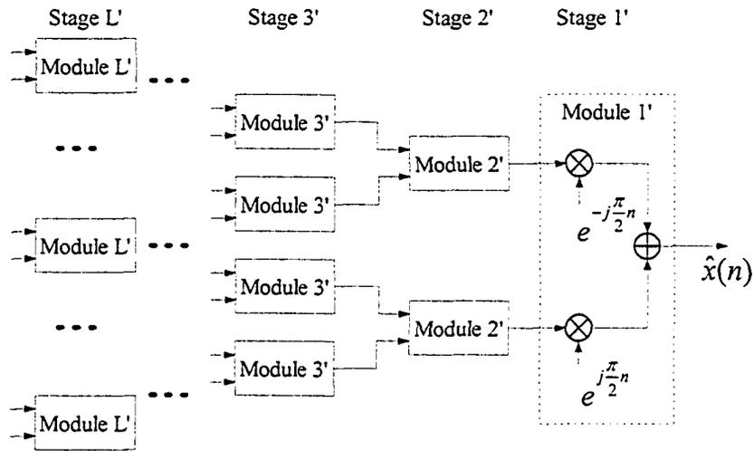
Figure 3.2: Multistage tree-structured synthesis filterbank
