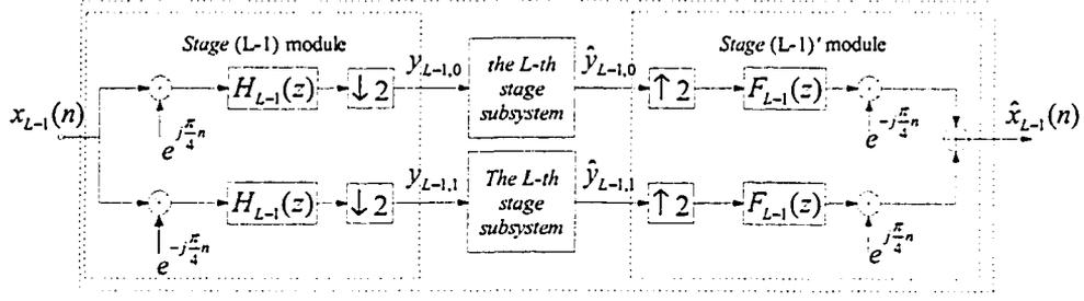
Figure 3.10: Detailed structure of  $(L - 1)$ -th subsystem
