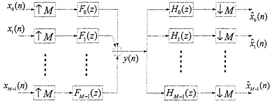
Figure 1.15:  $M$ -channel synthesis and analysis filterbanks for transmultiplexing
