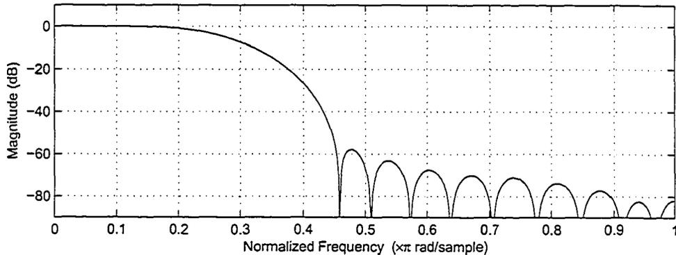
Figure 3.29: magnitude-frequency response of the optimized last-stage filter  $H_L(z)$
