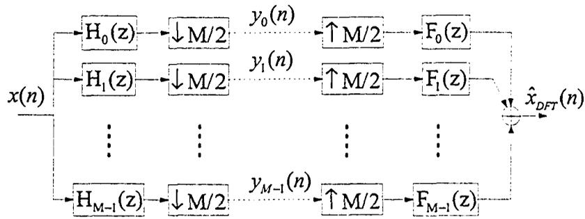
Figure 2.13: The  $M$ -channel Discrete Fourier Transform filterbank with  $M/2$ -fold decimation
