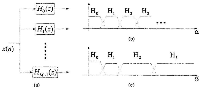
Figure 1.13:  $M$ -channel analysis filterbanks
