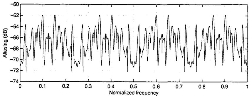
Figure 4.23: Aliasing function  $A(z)$  for the MDFT filterbank in Example 2
