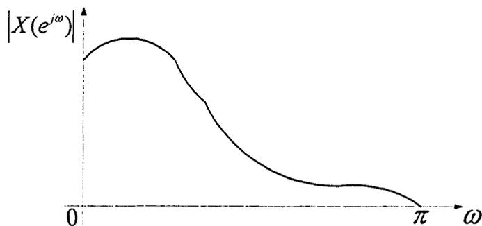
Figure 1.10: A signal with energy distribution concentrated in the low frequency region
