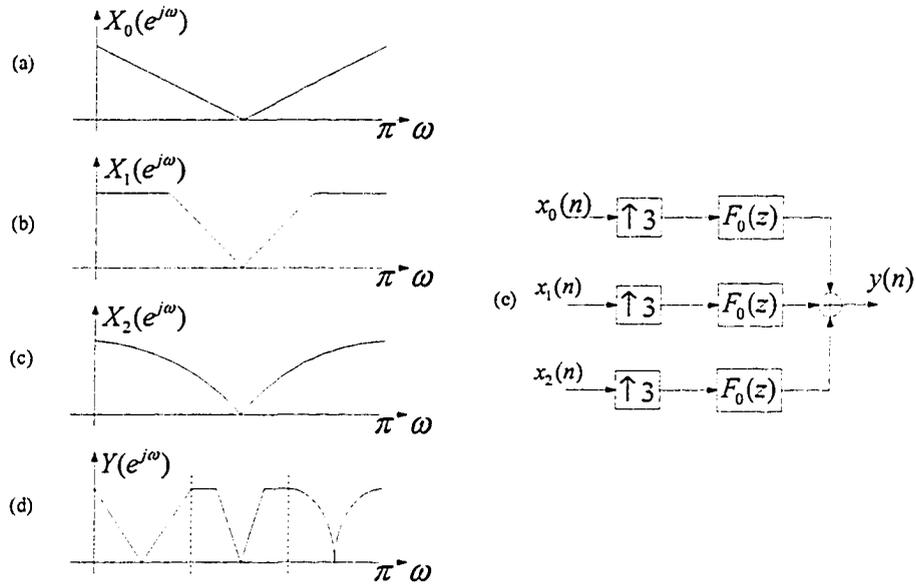
Figure 1.14: A 3-channel synthesis filterbank for transmultiplexing
