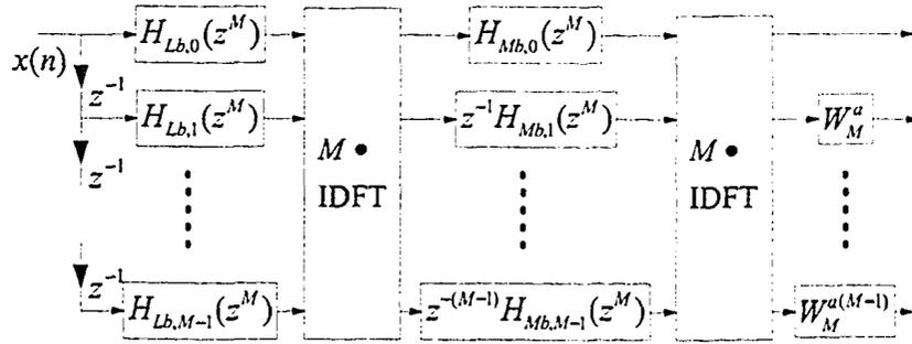
Figure 4.6: Realization of the analysis filters  $H_k(z)$  in terms of the polyphase components of  $H_{Lb}(z)$  and  $H_{Mb}(z)$  for a narrow-band FRM prototype digital filter  $P(z)$
