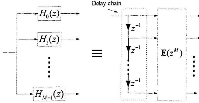
Figure 2.3: Type 1 polyphase representation of a  $M$ -channel analysis bank
