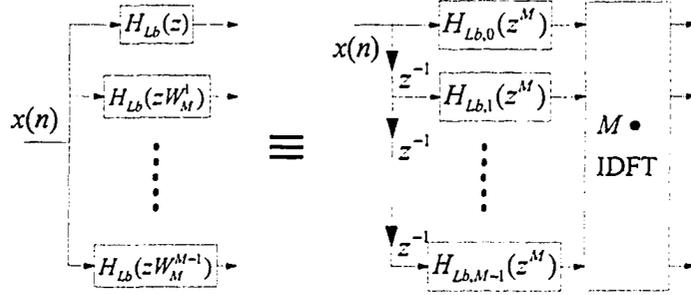
Figure 4.5: Realization of the filters  $H_{Lb}(zW_M^k)$  in terms of the polyphase components of  $H_{Lb}(z)$
