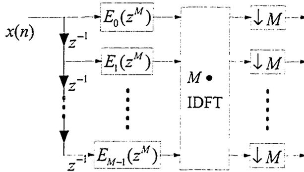
Figure 2.7: Polyphase representation of a maximally-decimated  $M$ -channel DFT analysis filterbank
