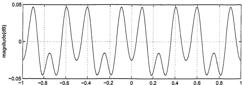
Figure 3.25: (a) The overall distortion of 2-Stage filterbank employing the windowing approach
