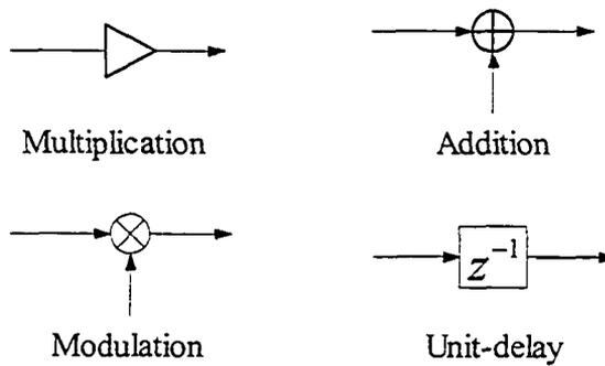
Figure 1.1: Building blocks in a single-rate DSP system
