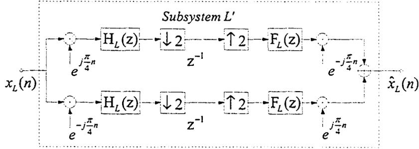
Figure 3.12: Alternative  $L$ -th subsystem
