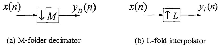
Figure 1.2: The decimator and interpolator building blocks
