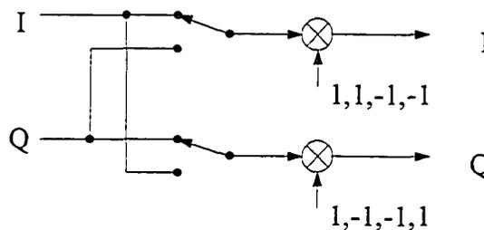
Figure 3.23: Simplified realization for real processing of complex signal sequences
