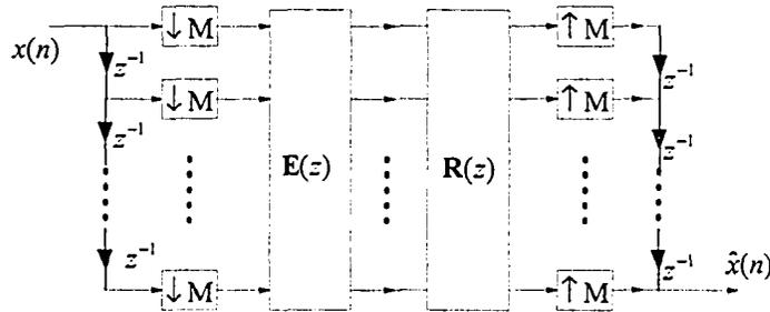
Figure 2.6: Simplified polyphase representation of an  $M$ -channel maximally-decimated filterbank
