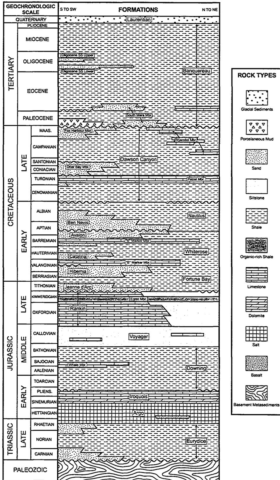
Figure 1.9: Lithostratigraphy for the entire sedimentary column hosted in the Jeanne d'Arc Basin. (Modified from Sinclair, 1988)
