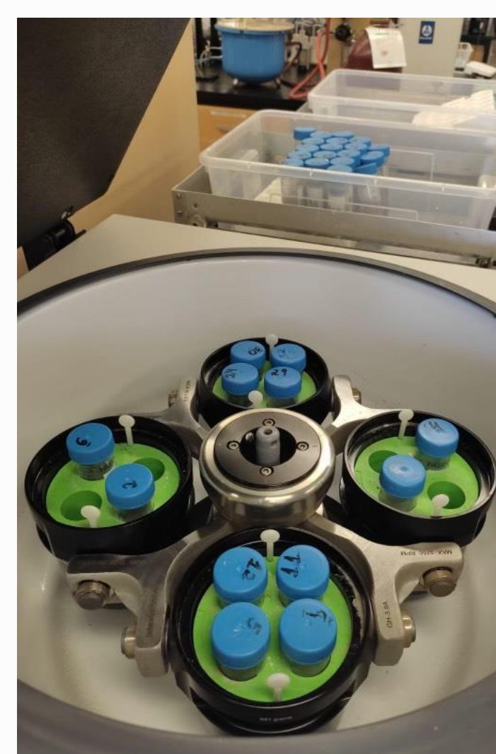
Figure 2: The centrifuge is used to separate the components of the Falcon tube. It spins at 3500 rpm for 30 minutes.
