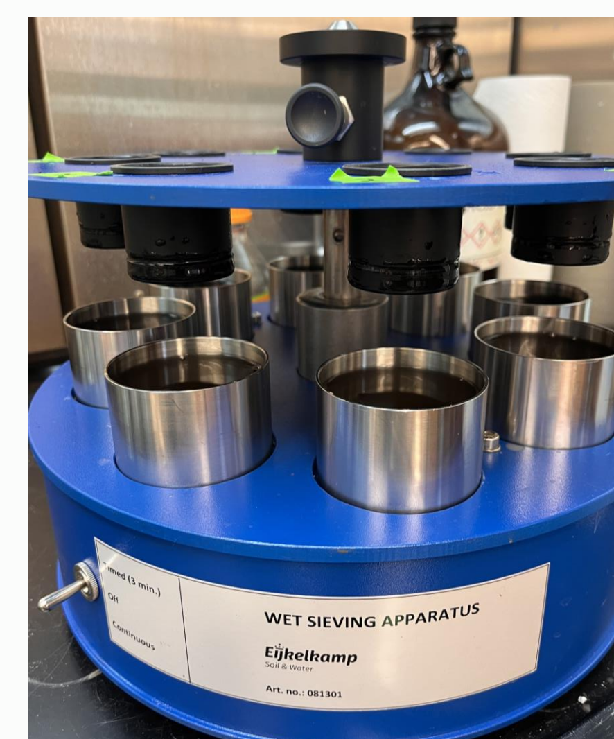
Figure 3: The wet sieving apparatus is used for most of the fractionation process. The black cylinders are the sieves which have a filter-like mesh on the bottom.
