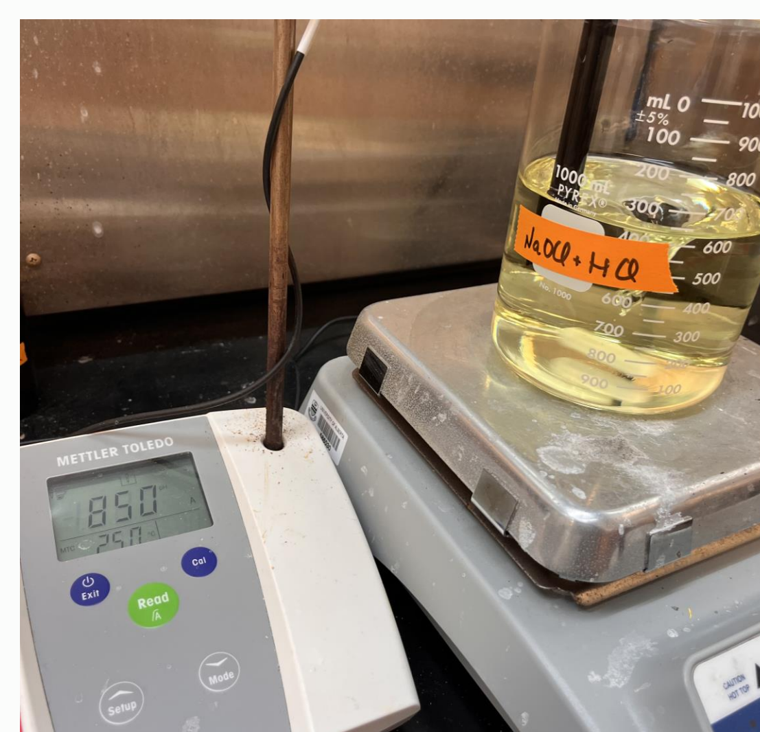
Figure 1: A solution of sodium hypochlorite (NaOCl) is mixed with hydrochloric acid using a magnetic stirring apparatus to lower the pH to 8.5. A pH probe (black rod) is placed into the solution to measure the pH precisely.
