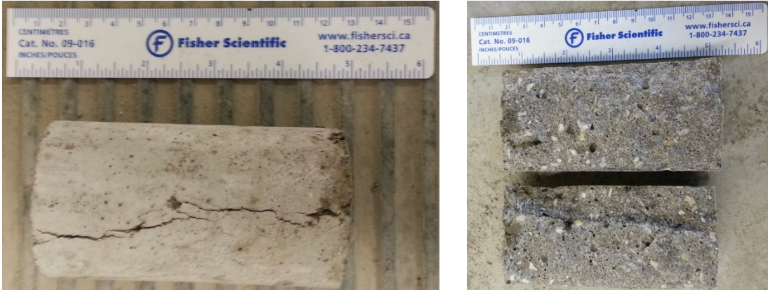
Figure 2-10 Typical failure shape of concrete sample in splitting tensile strength test
