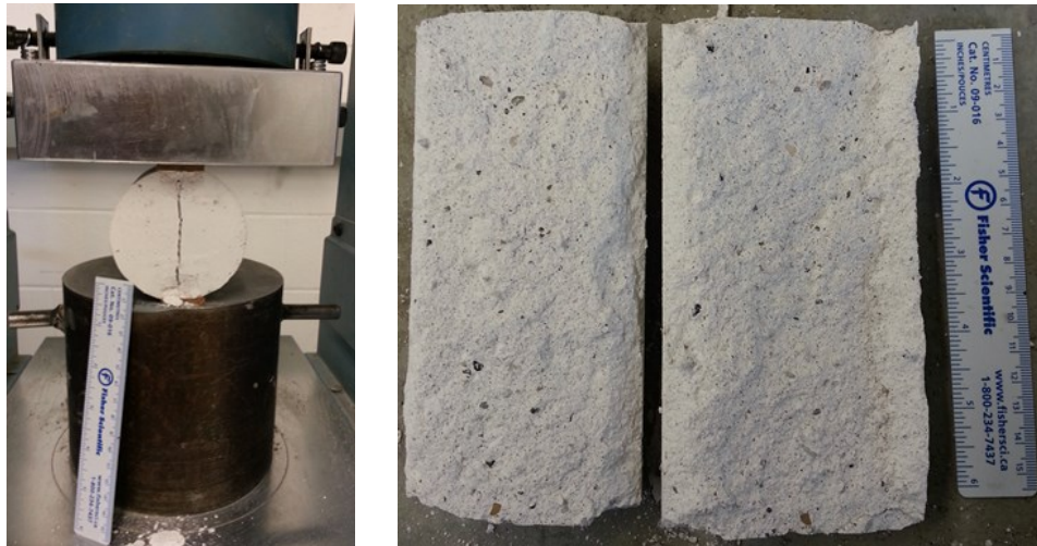
Figure 2-11 Typical failure shape of plaster sample in splitting tensile strength test
