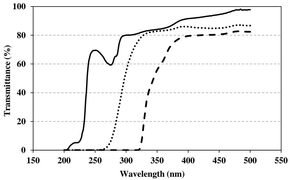
Figure 4-1: Transmittance spectra of a Pyrex® lid (dotted line), a PET bottle (dashed line) and Saran Wrap® (solid line).
