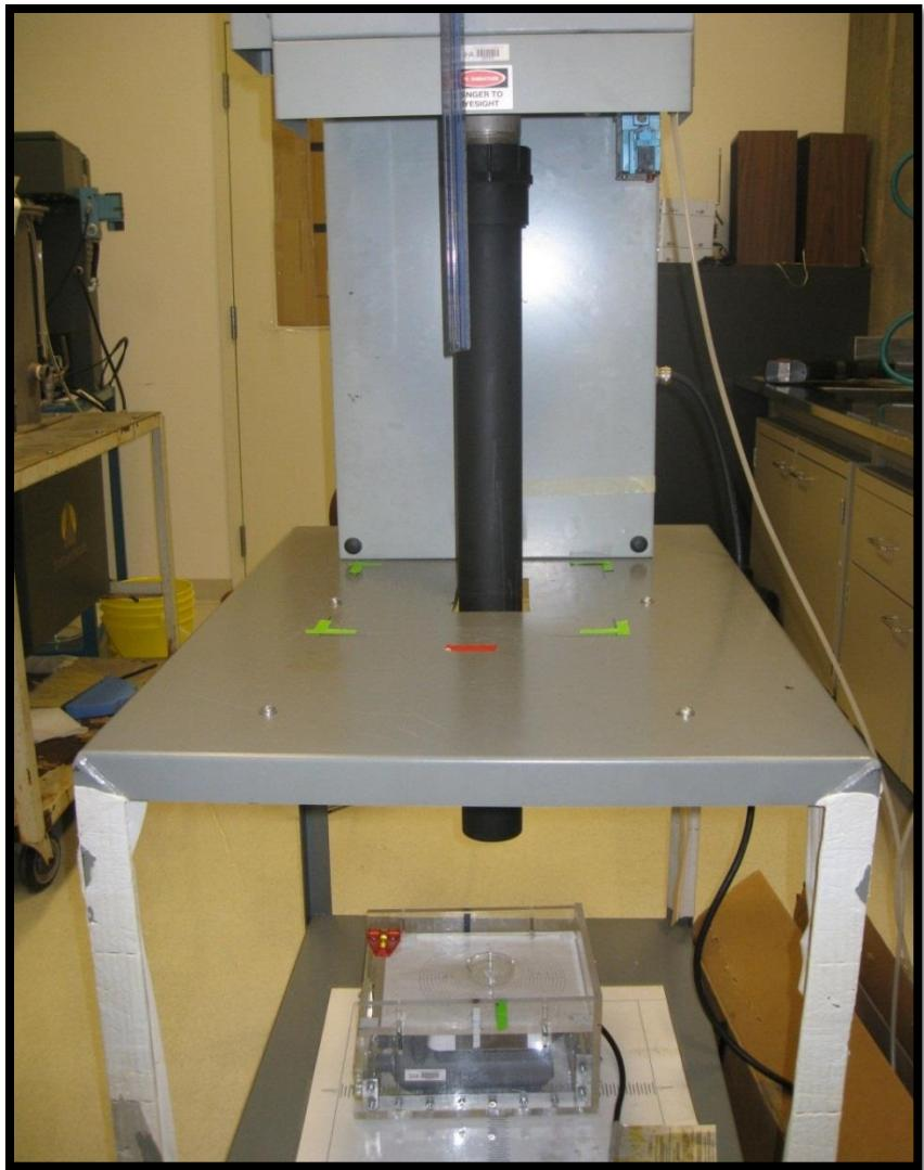
Figure 2-1: Diagram of the UV Collimated beam apparatus
