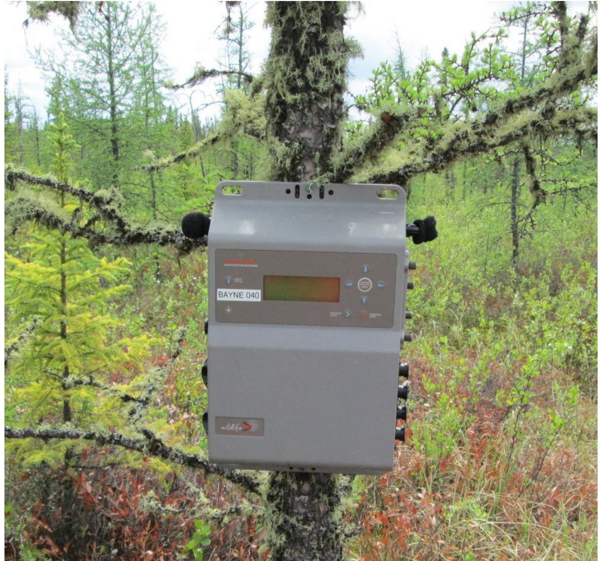
ARU Deployed in the field Photo: Bioacoustic Unit
