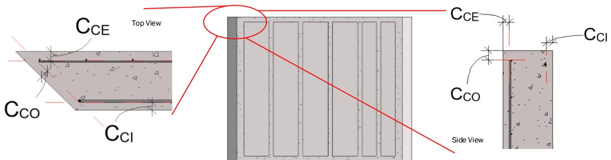
Figure 3-12. Concrete cover in top and section view of concrete panel.
