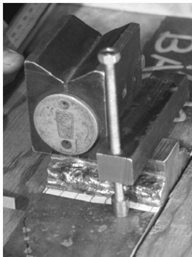
c) Place Measurement Head on Main Plate
