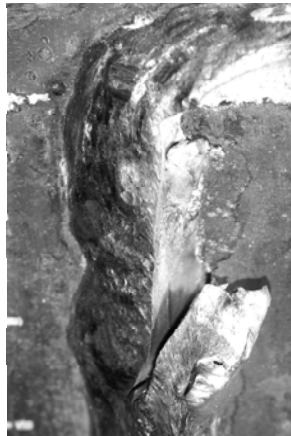
b) Close-Up of a Portion of the Fracture Surface that Has Been Distorted
