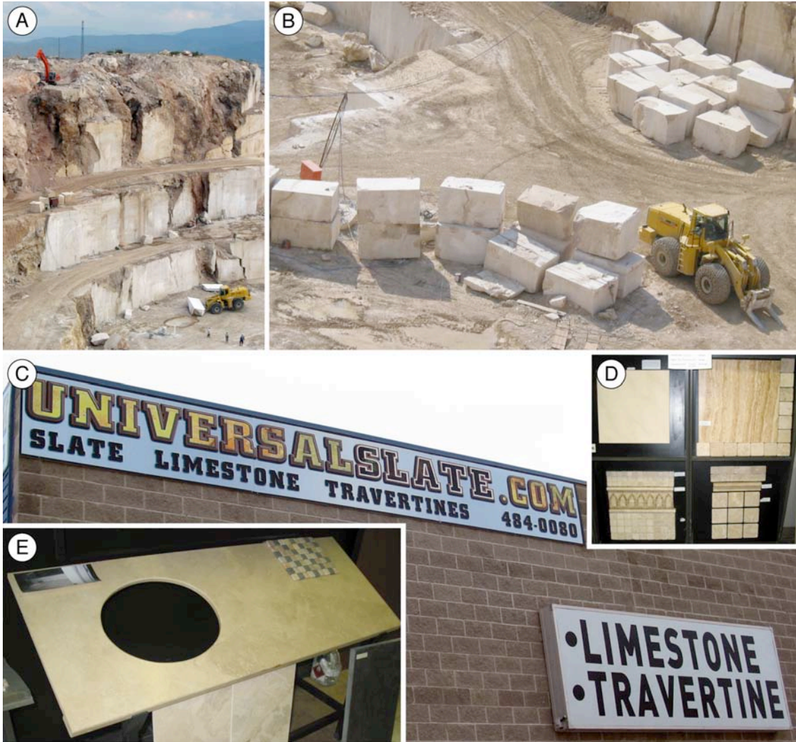
Fig. 1-3 Extraction and production of travertine to be used as facing stone. A) Three benches cut at the Ballik quarry near Denizli, Turkey. B) Each block weighs 20 to 30 tonnes and produces enough tile to cover an entire football field. C) Tile store in Edmonton on 170th street advertising travertine tile. D) Travertine tile samples. E) Travertine countertop.
