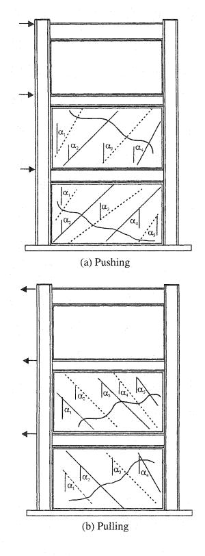
Figure 4.17: Tension field orientation in panels 1 and 2
