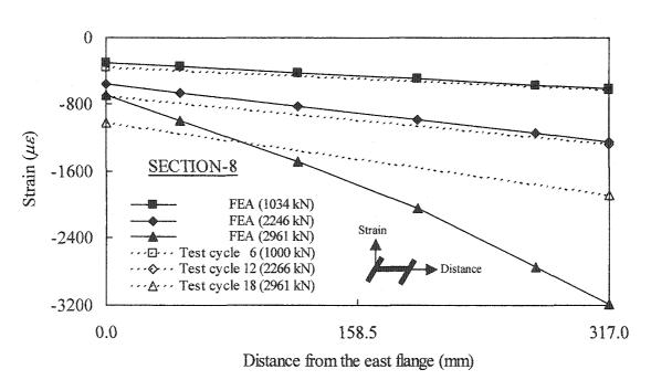
Figure 7.9: Strain distribution at section 8 in west column
