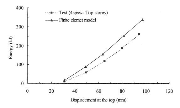
Figure 6.41: Energy dissipation as a function of displacement at the top
