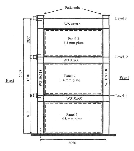
Figure 3.1: Schematic of three-storey steel plate shear wall
