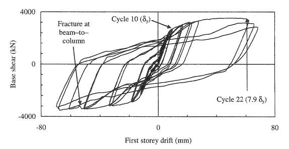
Figure 4.10: Base shear versus first storey drift
