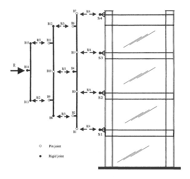
Figure 5.13: Loading frame for displacement control of the four-storey steel plate shear wall specimen
