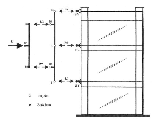
Figure 5.12: Loading frame for displacement control of the three-storey steel plate shear wall specimen
