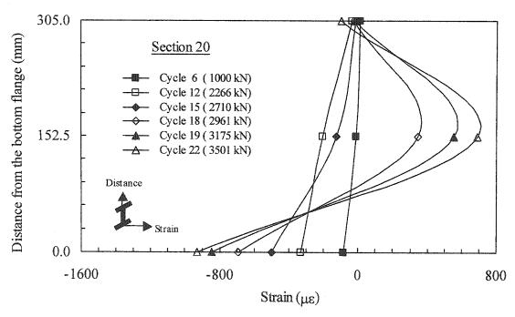
Figure 7.3: Strain distribution at section 20 in beam at level 2
