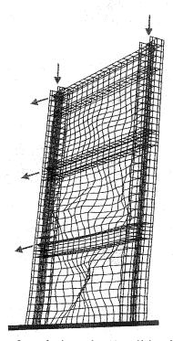
Figure 6.20: Deformed shape of steel plate shear wall loaded in negative 1-direction — Early stage of tension field redevelopment
