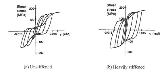
Figure 2.1: Hysteresis behaviour of steel plate shear walls (Takahashi et al., 1973)
