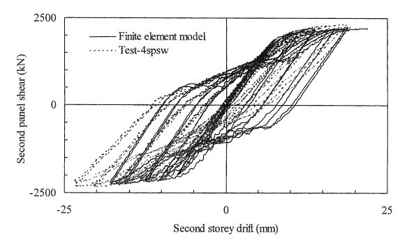
Figure 6.33: Comparison of finite element hysteresis analysis with test results—Panel 2
