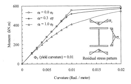
Figure 7.15: Effect of residual stresses on the moment versus curvature response for a W118×60
