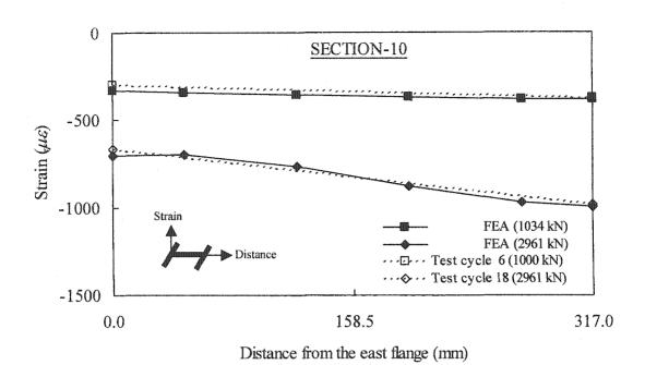
Figure 7.4: Strain distribution at section 10 in west column
