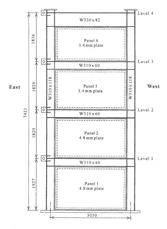
Figure 2.5: Four-storey steel plate shear wall tested by Driver et al. (1997)
