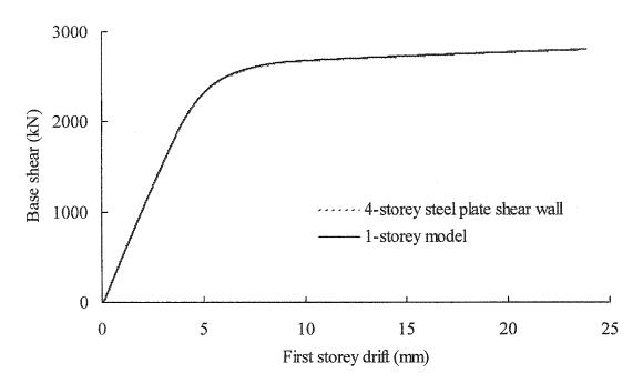
Figure 8.12: Base shear versus first storey drift obtained from the analysis of whole model and single storey model
