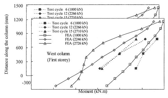
Figure 7.18: Bending moment diagram of the west column in the first storey
