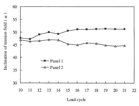
Figure 4.18 Average inclination of the tension field in the first and second panels
