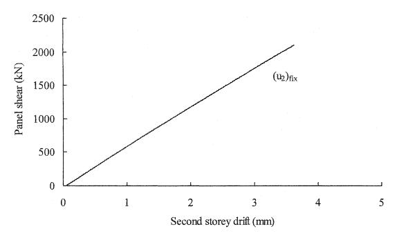
Figure 8.14: Panel shear versus storey drift obtained from single storey model of the second panel with fixed boundary condition
