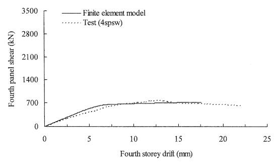
Figure 6.29: Monotonic finite element analysis compared with the envelope of the test cyclic response — Panel 4
