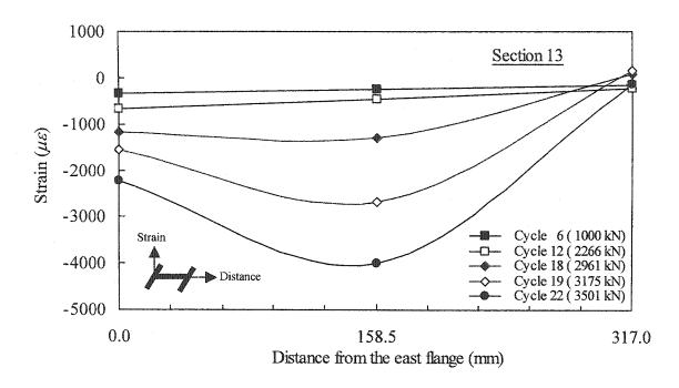
Figure 7.2: Strain distribution at section 13 in west column
