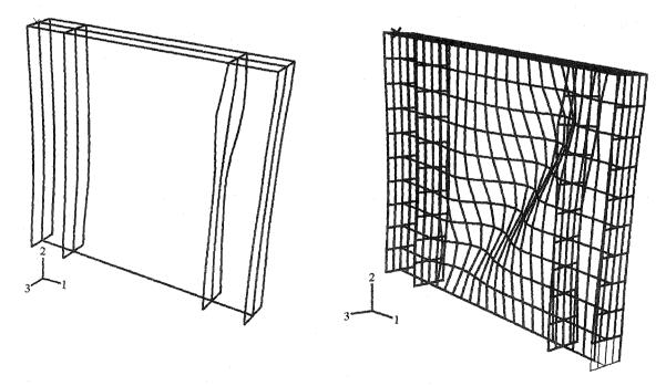
Figure 8.5: Column local buckling and deformation of model with  $\beta_1 = 0.7$
