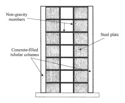
Figure 2.6: Steel plate shear wall system studied by Astaneh-Asl and Zhao (2002)
