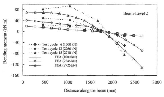
Figure 7.24: Bending moment diagram in the beam at level 2
