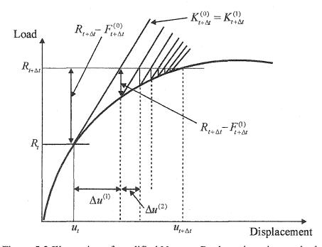
Figure 5.2 Illustration of modified Newton-Raphson iterative method
