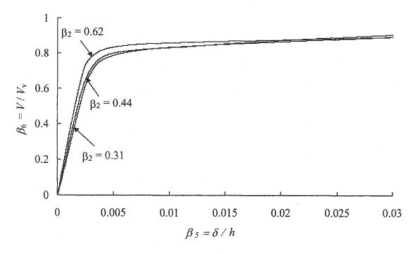
Figure 8.7: Effect of  $\beta_2$  on steel plate shear wall response
