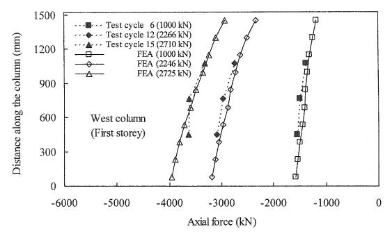
Figure 7.17: Axial force diagram of the west column in the first storey
