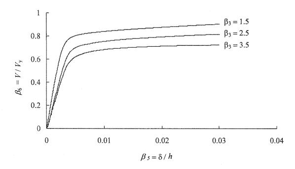
Figure 8.8: Effect of  $\beta_3$  on the normalized response of steel plate shear wall
