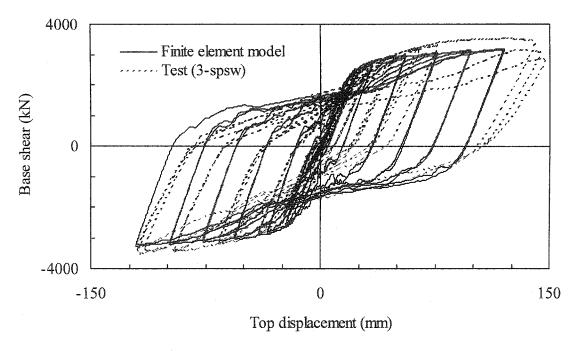
Figure 6.18: Comparison of finite element hysteresis analysis with test results— Top displacement
