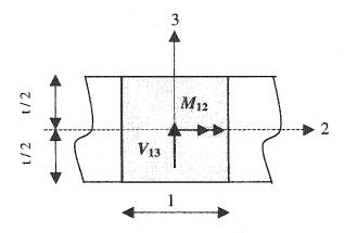
Figure A.1: Shell element subjected to bending and shear in the plane normal to direction 1.
