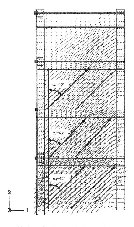
Figure 6.31: Vector plot of maximum in-plane principal stress at ultimate load—Mid-surface of shell elements
