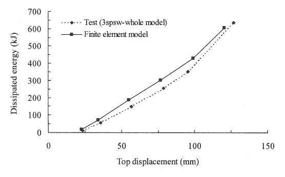
Figure 6.25: Energy dissipation as a function of displacement at the top
