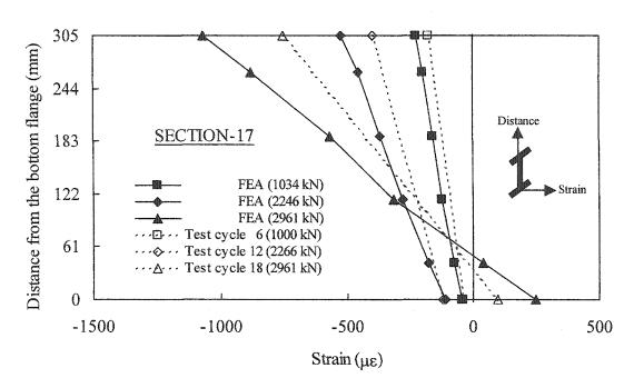
Figure 7.11: Strain distribution at section 17 in the beam at level 2
