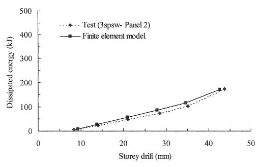
Figure 6.23: Energy dissipation as a function of drift level—Panel 2
