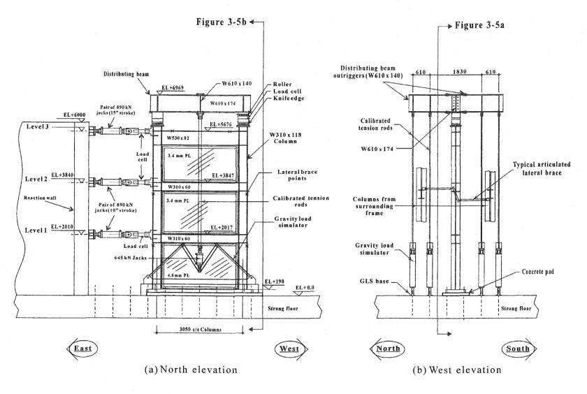
Figure 3.5: Three-storey steel plate shear wall test set up
