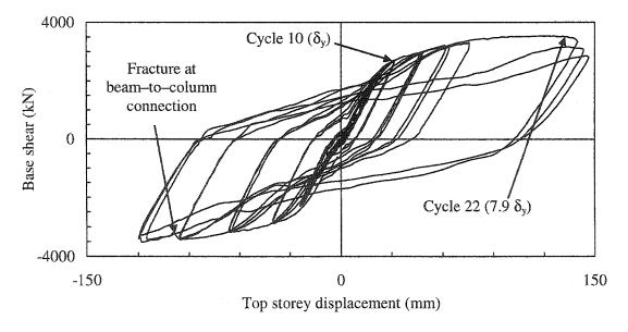
Figure 4.13: Base shear versus top storey displacement
