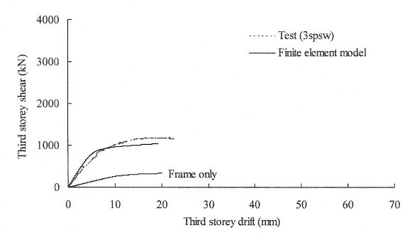
Figure 6.8: Monotonic finite element analysis compared with the envelope of the test cyclic response — Panel 3
