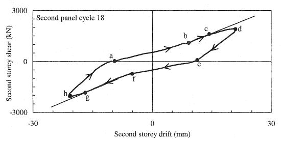
Figure 4.14: Typical hysteresis curve, 2<sup>nd</sup> panel, cycle 18
