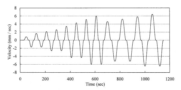
Figure 6. 11: History of horizontal velocity applied to node B7 on loading frame
