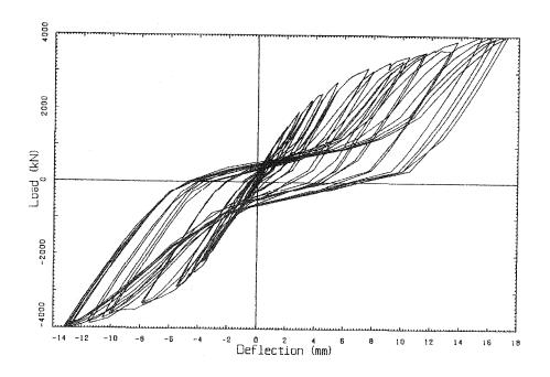
Figure 2.4: Hysteresis behaviour of specimen tested by Tromposch and Kulak (1987)
