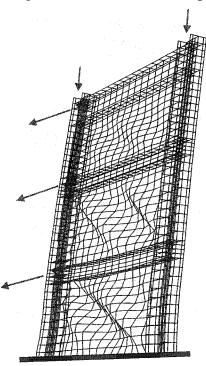
Figure 6.21: Deformed shape of steel plate shear wall loaded in negative 1-direction — Tension field fully redeveloped
