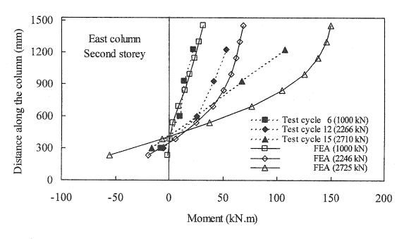
Figure 7.22: Bending moment diagram of the east column in the second storey
