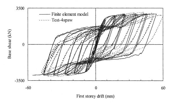
Figure 6.32: Comparison of finite element hysteresis analysis with test results—Panel 1
