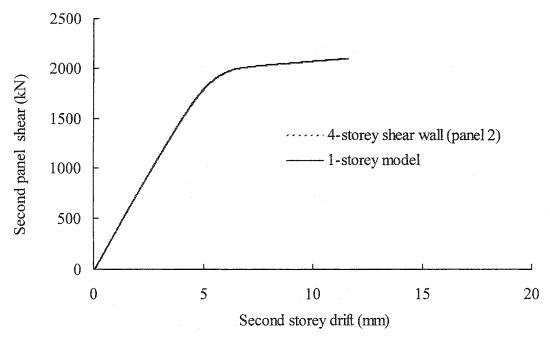
Figure 8.15: Panel shear versus storey drift obtained from the analysis of whole model and single storey model of the second panel
