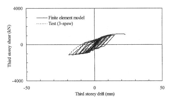
Figure 6.17: Comparison of finite element hysteresis analysis with test results—Panel 3
