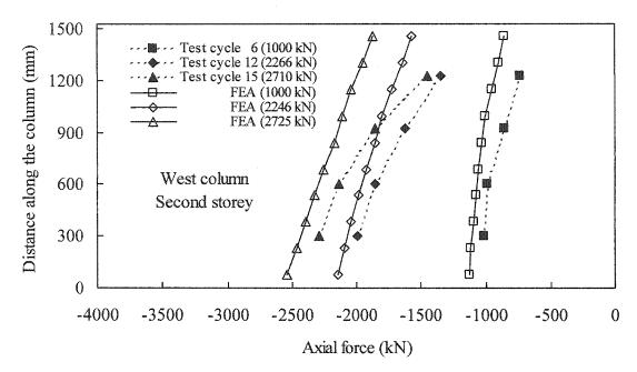
Figure 7.19: Axial force diagram of the west column in the second storey
