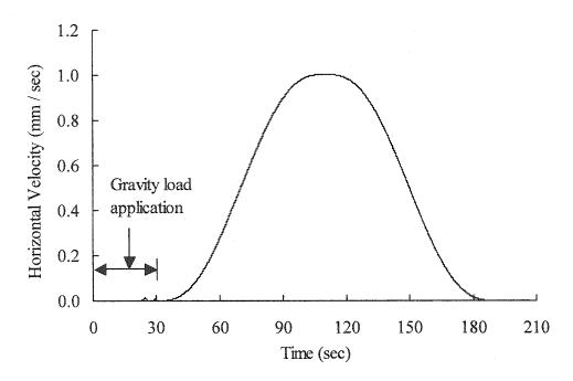
Figure 6.2: Velocity history for node B7 in the pushover analysis of the three-storey steel plate shear wall
