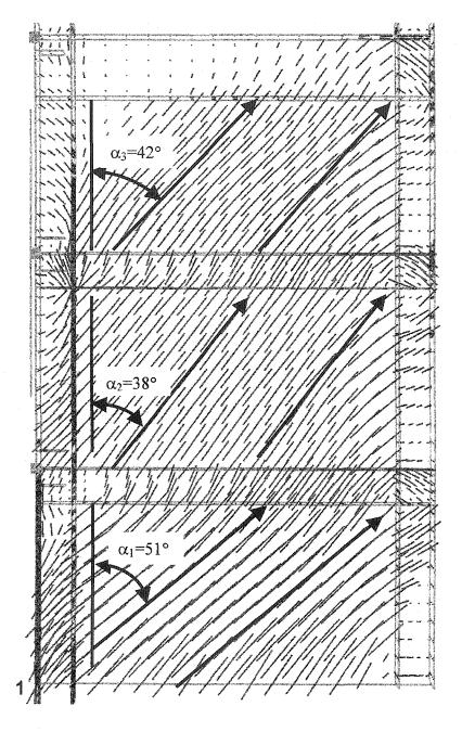
Figure 6.10: Vector plot of maximum in-plane principal stress at ultimate load—Mid surface of shell elements
