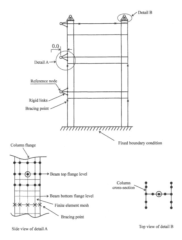
Figure 5.10: Boundary and loading conditions for the finite element model
