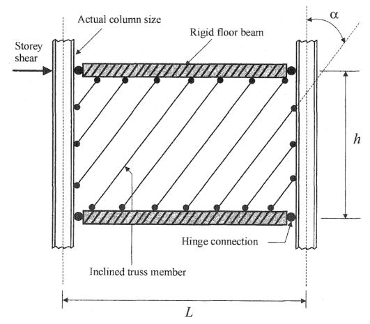
Figure 2.2: Strip model proposed by Thorburn and Kulak (1983)
