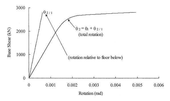
Figure 8.16: Rotation of the second floor
