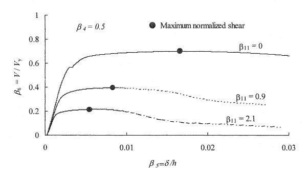
Figure 8.22: Normalized response at  $\beta_4$  equal to 0.5 and various  $\beta_{II}$  parameter
