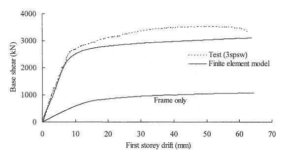
Figure 6.6: Monotonic finite element analysis compared with the envelope of the test cyclic response — Panel 1
