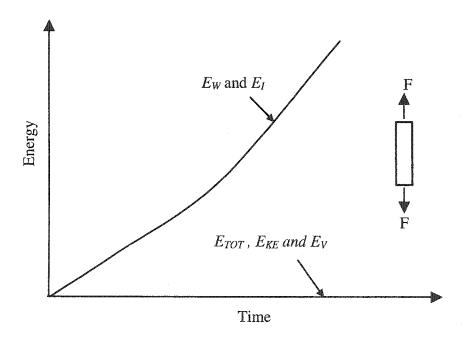
Figure 5.6: Energy history for quasi-static tensile test
