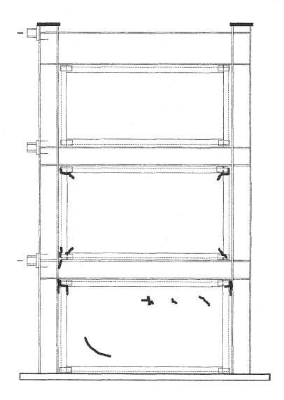
Figure 4.9: Location of tears in the test specimen at the end of the test (north side)
