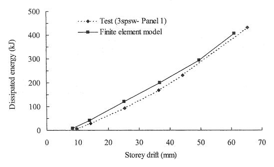
Figure 6.22: Energy dissipation as a function of drift level—Panel 1
