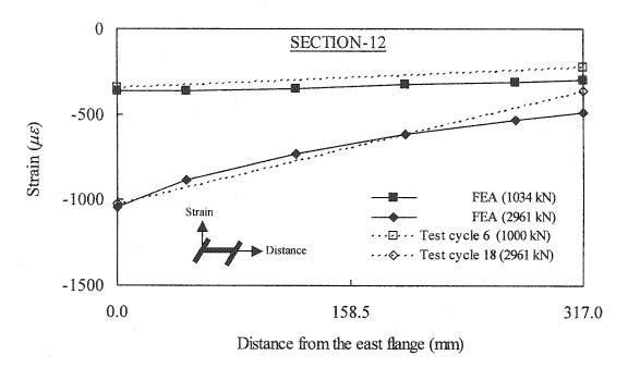
Figure 7.6: Strain distribution at section 12 in west column
