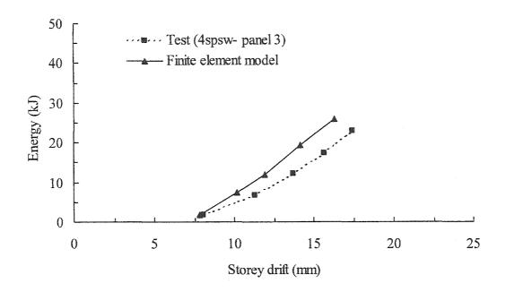
Figure 6.39: Energy dissipation as a function of drift level—Panel 3
