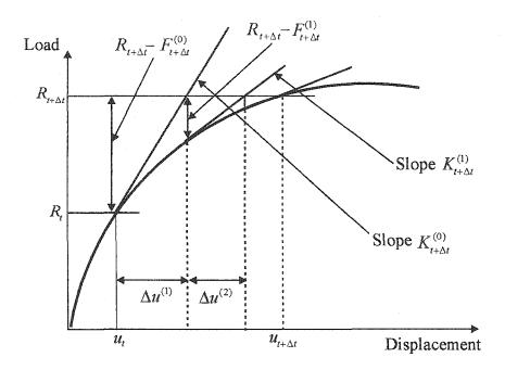
Figure 5.1: Illustration of Newton-Raphson iterative method
