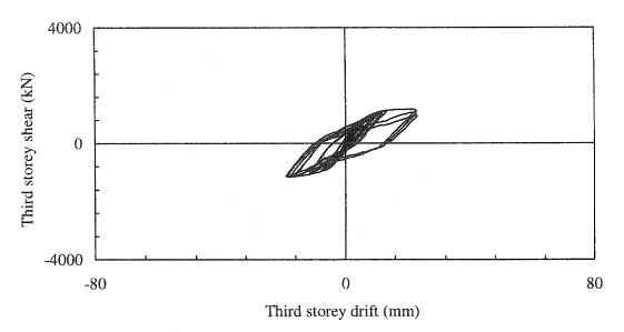
Figure 4.12: Third storey shear versus third storey drift
