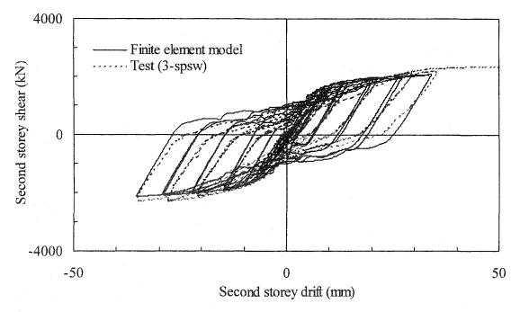
Figure 6.16: Comparison of finite element hysteresis analysis with test results—Panel 2
