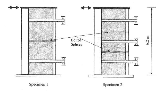
Figure 2.7: Specimens tested by Astaneh-Asl and Zhao (2002)
