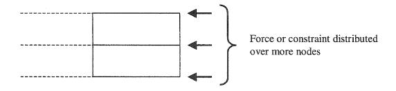
(c) Improved deformation pattern with distributed force or constraint
