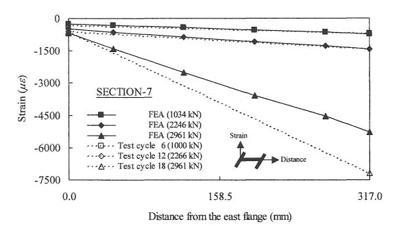
Figure 7.8: Strain distribution at section 7 in west column
