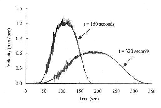
Figure 6.5: Top storey velocity history during a pushover analysis of the three-storey steel plate shear wall for two different time periods
