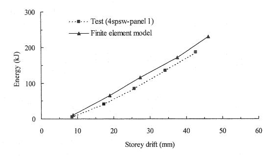
Figure 6.37: Energy dissipation as a function of drift level—Panel 1
