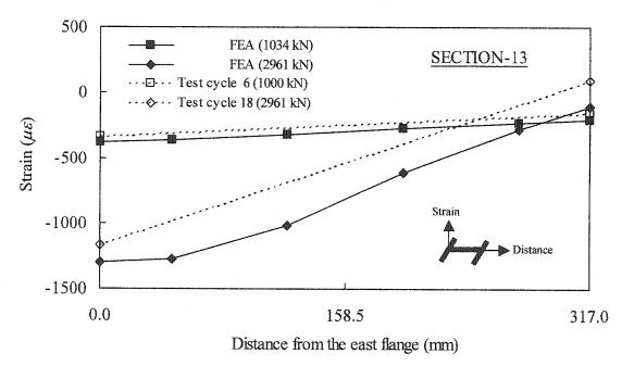
Figure 7.7: Strain distribution at section 13 in west column
