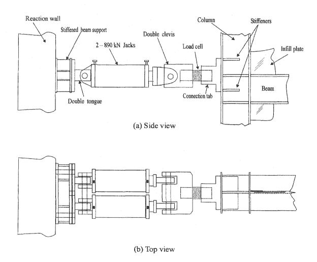
Figure 3.7: Detail of connection of hydraulic jacks to the test specimen
