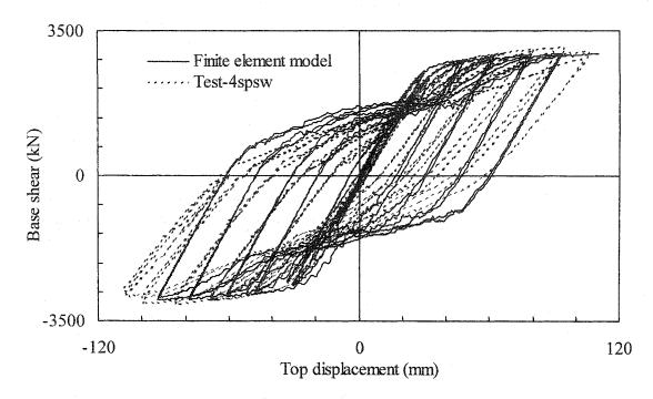
Figure 6.36: Comparison of finite element hysteresis analysis with test results— Displacement at the top
