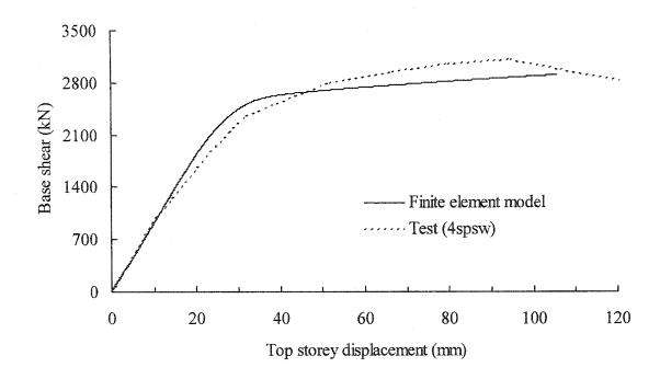
Figure 6.30: Monotonic finite element analysis compared with the envelope of the test cyclic response — Top displacement
