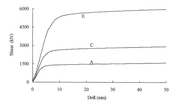
Figure 8.2: Base shear versus drift for three models with similar  $\beta$ -parameters
