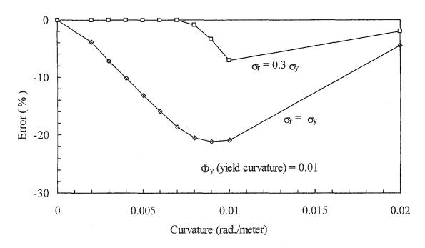
Figure 7.16: Error introduced when residual stresses are ignored in moment calculation
