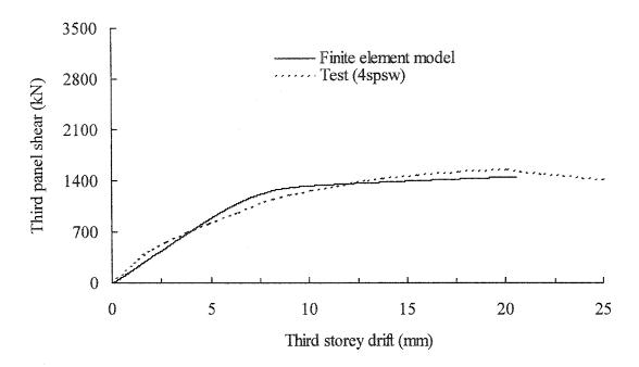
Figure 6.28: Monotonic finite element analysis compared with the envelope of the test cyclic response — Panel 3
