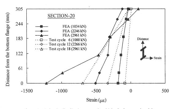
Figure 7.14: Strain distribution at section 20 in the beam at level 2
