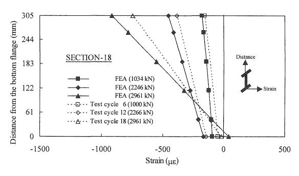
Figure 7.12: Strain distribution at section 18 in the beam at level 2
