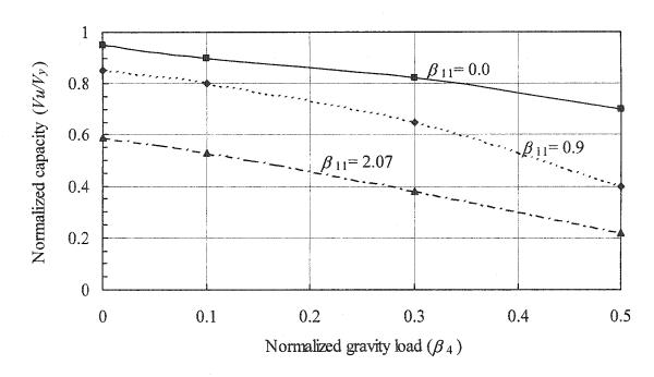
Figure 8.19: Effect of  $\beta_4$  and  $\beta_{11}$  on shear wall panel capacity
