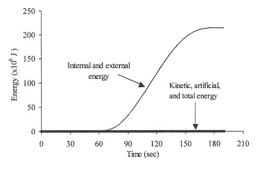
Figure 6.3: Energy history of the pushover analysis of the three-storey steel plate shear wall
