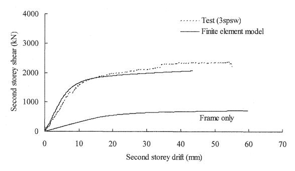
Figure 6.7: Monotonic finite element analysis compared with the envelope of the test cyclic response — Panel 2
