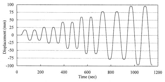
Figure 6.12: History of horizontal displacement at node B7 on loading frame
