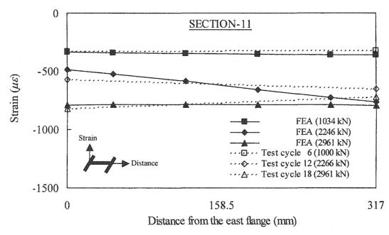
Figure 7.5: Strain distribution at section 11 in west column
