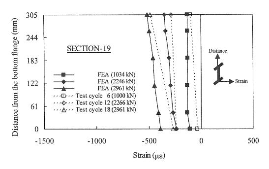
Figure 7.13: Strain distribution at section 19 in the beam at level 2
