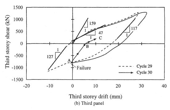
Figure 4.15: Response of four-storey steel plate shear wall specimen (cycles 29 and 30)
