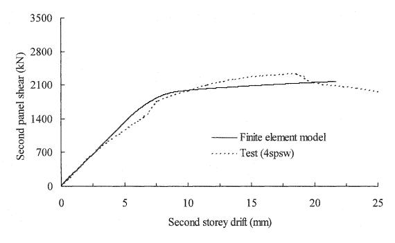
Figure 6.27: Monotonic finite element analysis compared with the envelope of the test cyclic response — Panel 2
