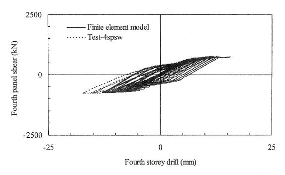
Figure 6.35: Comparison of finite element hysteresis analysis with test results—Panel 4
