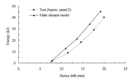
Figure 6.38: Energy dissipation as a function of drift level—Panel 2
