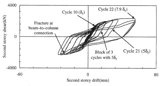
Figure 4.11: Second storey shear versus second storey drift
