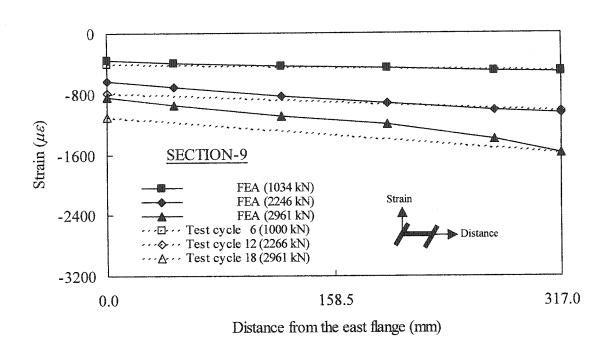
Figure 7.10: Strain distribution at section 9 in west column
