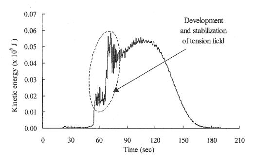
Figure 6.4: History of kinetic energy of the pushover analysis of the three-storey steel plate shear wall
