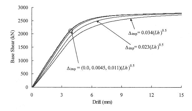
Figure 8.9: Effect of imperfection magnitude on the behaviour of a steel plate shear wall panel
