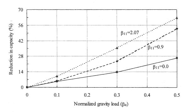
Figure 8.20: Effect of  $\beta_4$  and  $\beta_{II}$  on reduction of shear wall panel capacity
