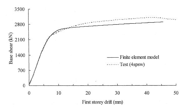
Figure 6.26: Monotonic finite element analysis compared with the envelope of the test cyclic response — Panel 1
