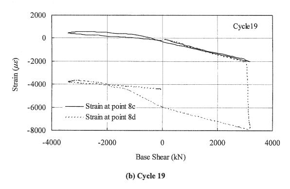
Figure 7.1: Strain versus base shear at points c and d of section 8
