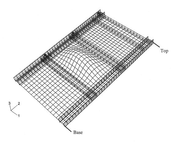
Figure 6.1: First vibration mode of the three-storey steel plate shear wall
