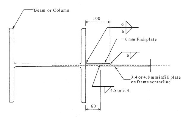
Figure 3.3: Fish plate detail used for connection of infill plate to the frame
