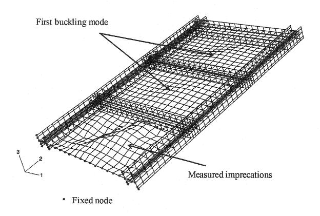
Figure 5.9: Imperfection shape used in finite element model (magnification factor = 5.0)
