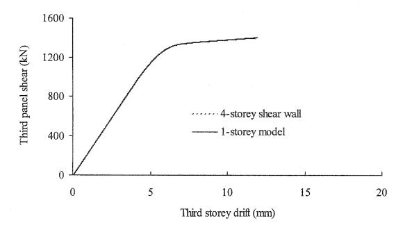
Figure 8.17: Third storey shear versus third storey drift obtained from the analysis of whole model and single storey model of the third panel
