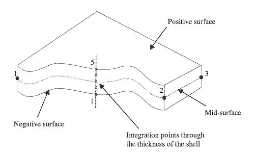
Integration points through the thickness of shell element
