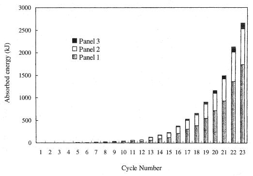
Figure 4.16: Cumulative energy absorbed by each panel through the test
