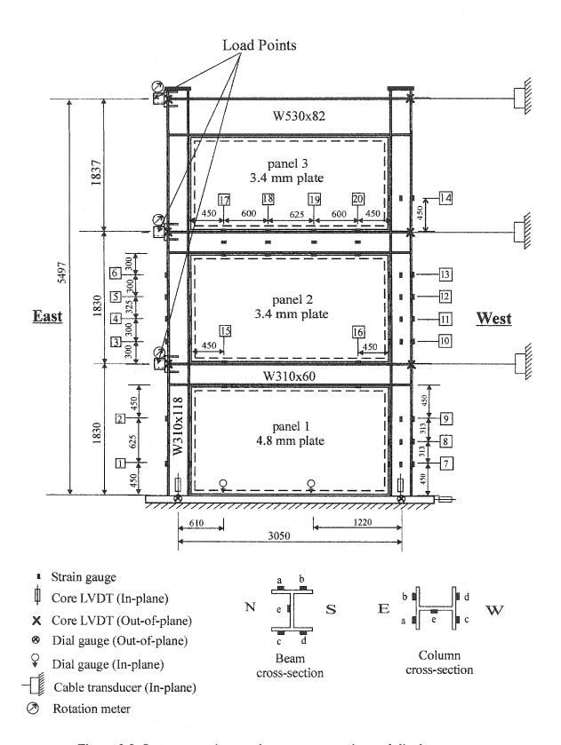
Figure 3.9: Instrumentation used to measure strains and displacements
