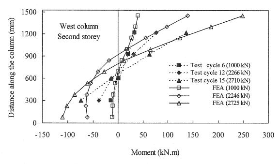
Figure 7.20: Bending moment diagram of the west column in the second storey
