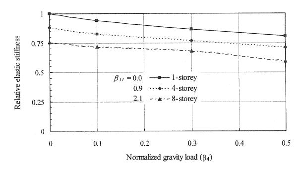
Figure 8.18: Elastic stiffness of the panel versus  $\beta_4$  at different  $\beta_{II}$  parameters
