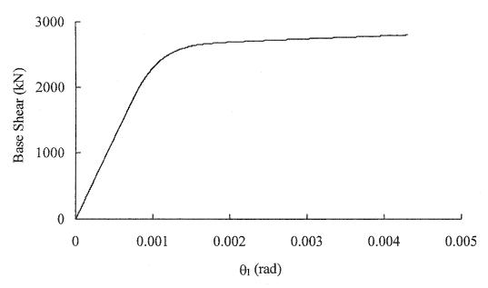
Figure 8.13: Rotation of the first floor obtained from the analysis of a single storey model of the first panel
