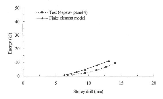
Figure 6.40: Energy dissipation as a function of drift level—Panel 4
