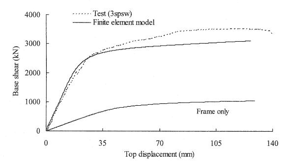
Figure 6.9: Monotonic finite element analysis compared with the envelope of the test cyclic response — Top displacement
