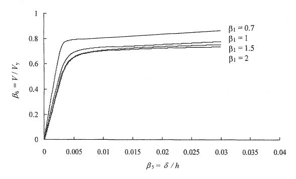
Figure 8.6: Normalized response for different aspect ratios (if column local buckling prevented)
