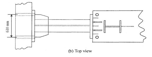
Figure 3.8: Schematic of in-plane bracing at the base of specimen
