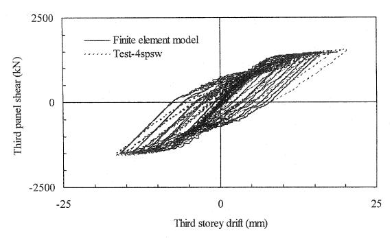
Figure 6.34: Comparison of finite element hysteresis analysis with test results—Panel 3
