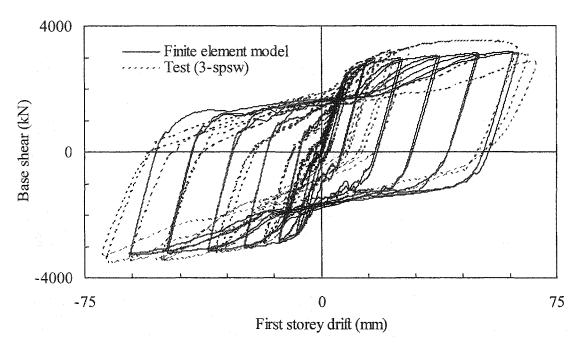
Figure 6.15: Comparison of finite element hysteresis analysis with test results—Panel 1
