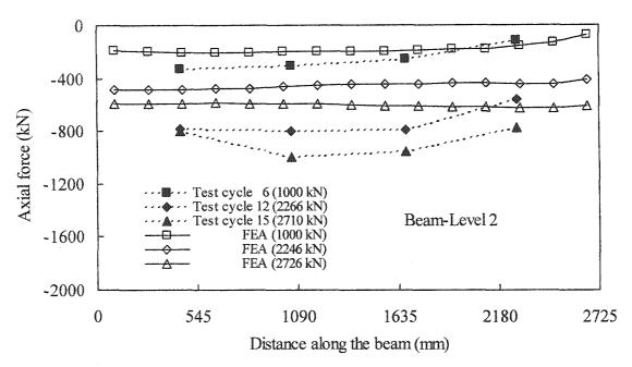
Figure 7.23: Axial force diagram in the beam at level 2
