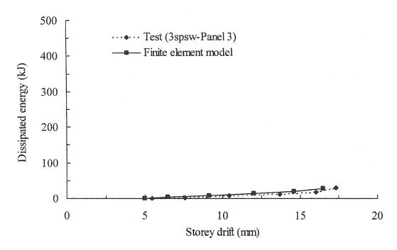
Figure 6.24: Energy dissipation as a function of drift level—Panel 3
