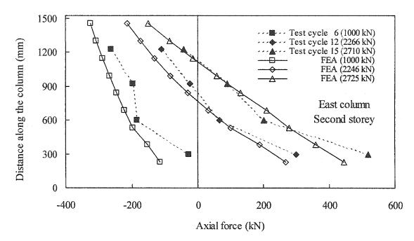
Figure 7.21: Axial force diagram of the east column in the second storey
