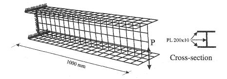
(a) Finite element mesh with load and boundary condition
