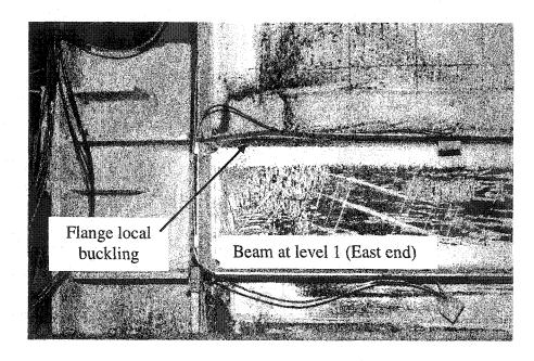
Figure 4.4: Initiation of flange local buckling – beam at level 1, east end (cycle 20)
