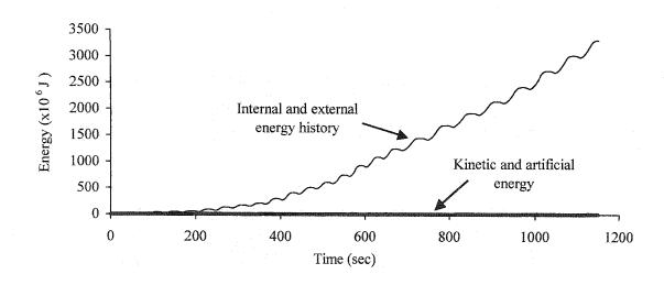
Figure 6.14: Energy history in cyclic analysis of the three-storey steel plate shear wall
