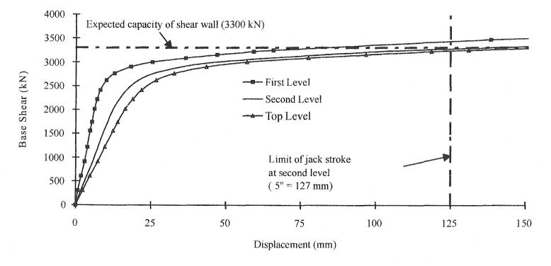
Figure 3.4: Preliminary finite element analysis of test specimen
