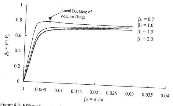
Figure 8.4: Effect of aspect ratio parameter,  $\beta_1$ , on behaviour of steel plate shear wall
