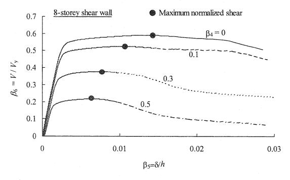
Figure 8.21: Normalized response of the first panel of an eight-storey shear wall at various  $\beta_4$  parameter
