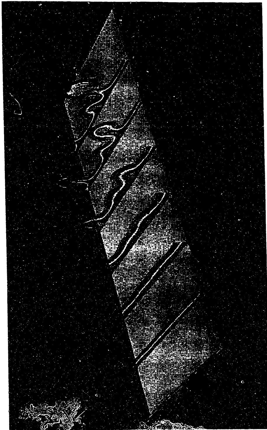
FIGURE 4.20. Contours of the streamwise velocity u_\theta of the Görtler vortices in figure 4.19 are shown in cross-stream planes from x = 0.0384 to 0.96 m with \Delta x = 0.1536 m. The concave wall is shown as a flat plate and the flow proceeds downstream from left to right.
