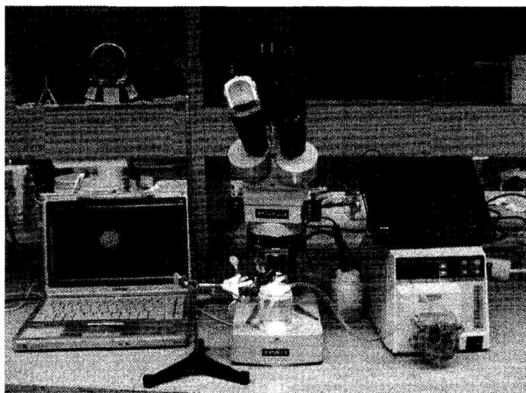
Figure 3-2 Experimental setup for visualization of bitumen (oil)-mineral adhesion.
