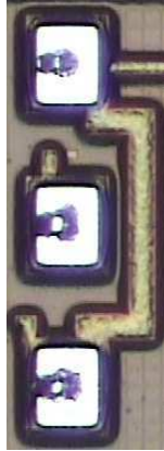
Figure 3.31: Die photographs of the RF pads designed for de-embedding.
