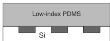
When the high-index PDMS has partially set, pour on the low-index PDMS and bake til set.
