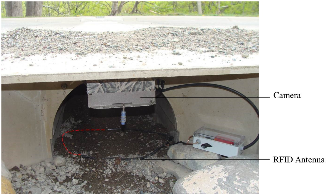
Figure 2.3 Photograph of an RFID antenna and camera in its protective box at the entrance of a tunnel. The red dashed line shows where the antenna is buried beneath the substrate. Cameras operated on a motion-detection setting 24 h each day and on a timed interval setting from 0600 h – 2100 h. Antennas scanned every 4 s, 24 h each day.
