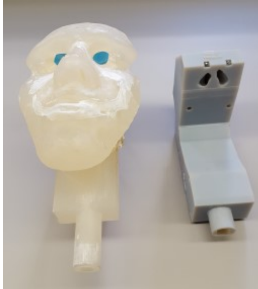
Figure 2-3: Example MRI-based replica (left) and CT-based replica (right).
