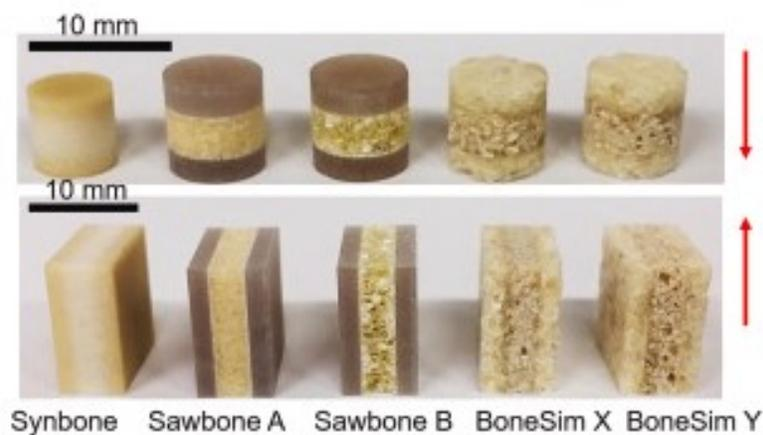
**Figure 10.** Three commercially available bone surrogates. A, B, X, Y correspond to different densities used by Brown et al. The red arrows correspond to the two different loading conditions applied, transverse (top arrow) and longitudinal (bottom arrow). **Image source: (Brown et al., 2019) Copyright permissions from Elsevier has been granted (license number: 5395490184561)<sup>1</sup>**
