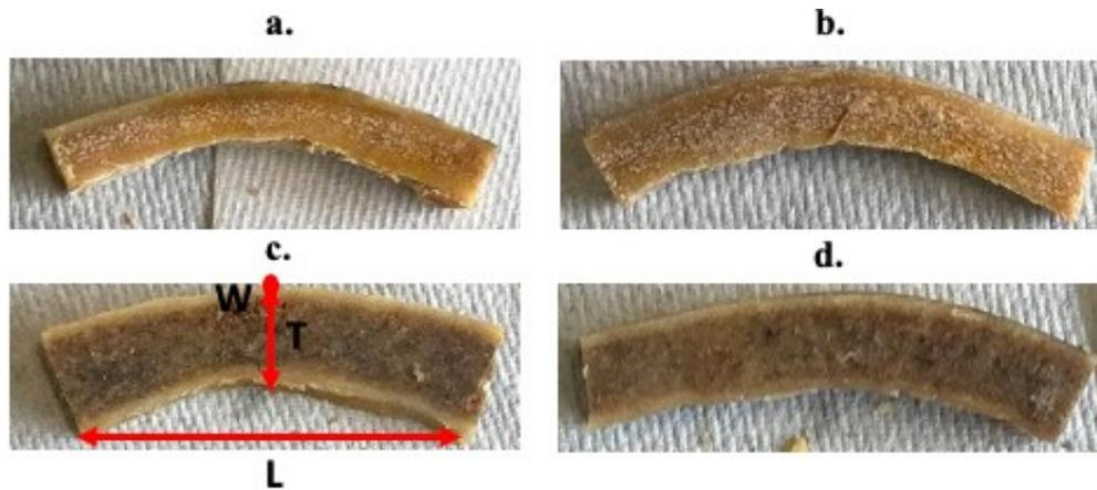
**Figure 2.** Example images of a male frontal (a.), male parietal (b.), female frontal (c.), and female parietal (d) calvarium specimen. *L*, *W* (into the page) and *T* correspond to the location of where length, width, and thickness dimensions were measured respectively at the center of each specimen using digital calipers.
