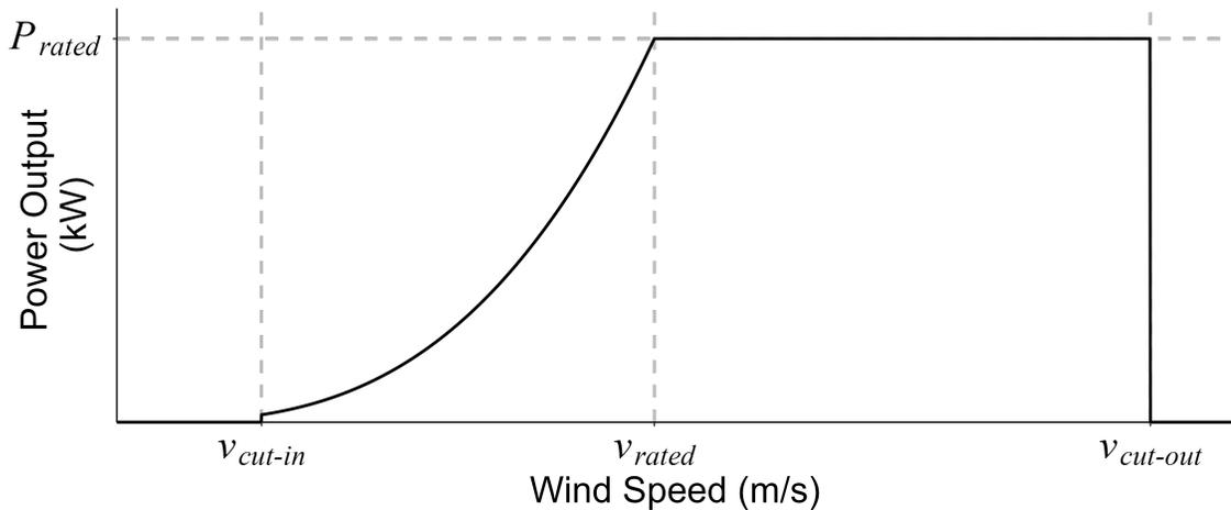
Figure 2.3: Typical wind turbine power curve.
