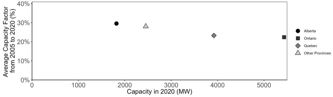
Figure 3.1: Average capacity factors by province with the installed wind capacity in 2020.
