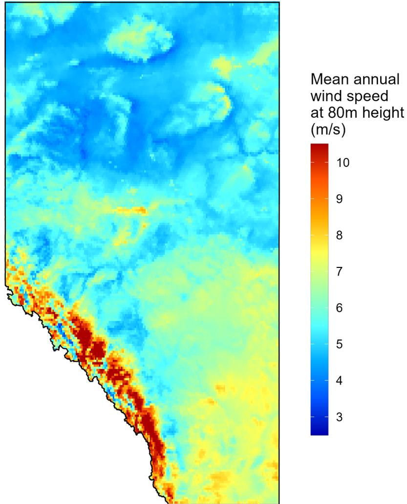
Figure 2.1: Annual mean wind speeds at 80 m above the ground. Ideal wind speeds shown in green with areas with wind speeds above the cut-out speed or below the cut-in speed for wind turbines shown in red. Source: Canada Wind Atlas [27].
