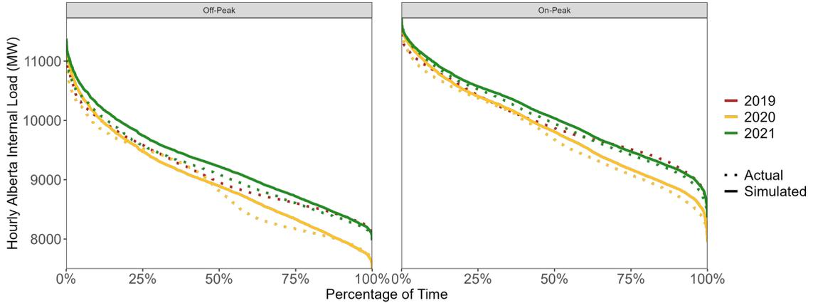
Figure 4.2: Simulated versus historic load duration curve [54]
