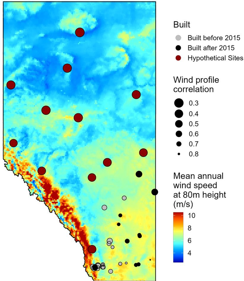
Figure 3.3: Map of Alberta showing the correlation between wind speed profiles at existing wind farm locations and potential locations identified for this research.
