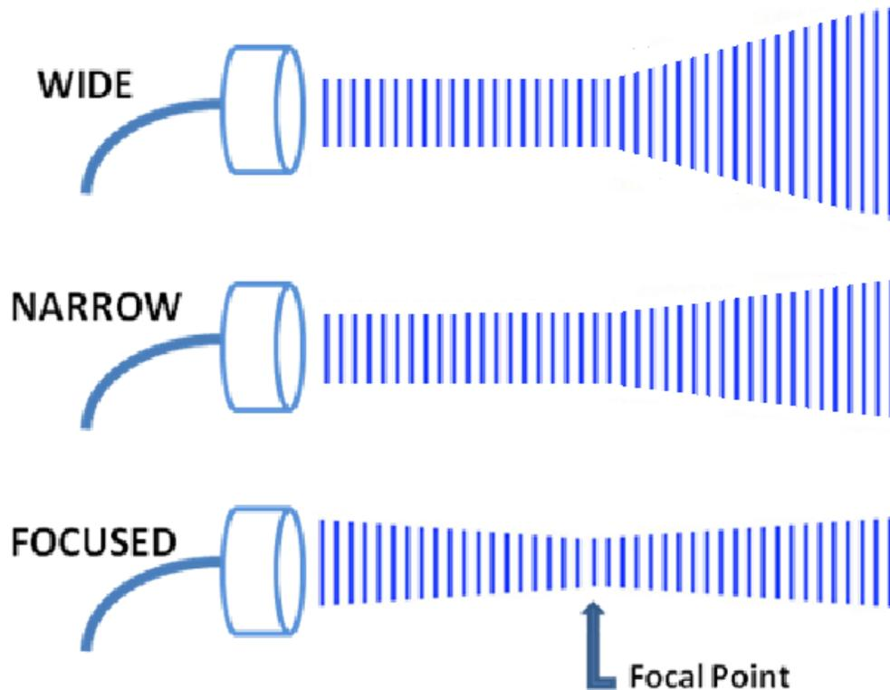
Figure 1.2 - The difference between ultrasound beam profile
