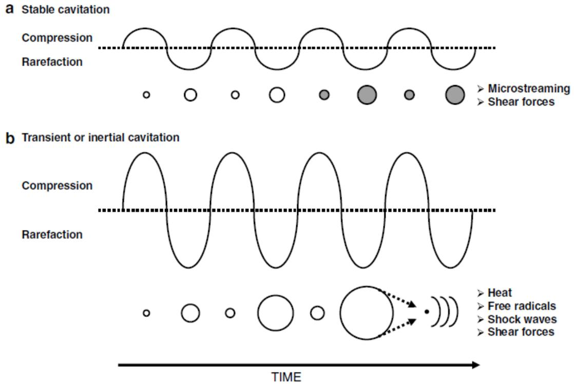
Figure 1.3 - Schematic illustrating of (a) Stable cavitation and (b) Inertial cavitation [64]
