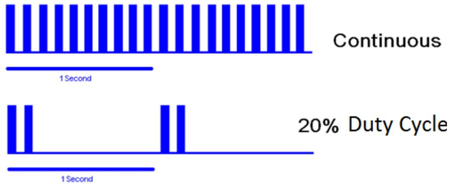
Figure 1.1 - The graphic representation of the difference in between Continuous ultrasound wave (Top) and Pulsed ultrasound wave with a 20% Duty cycle (Bottom)
