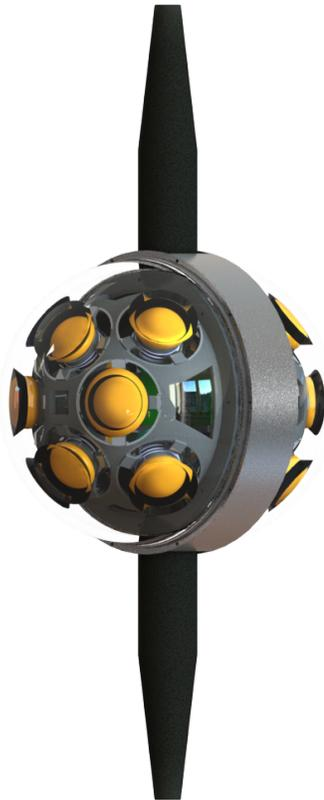
Figure 3.5: Digital Optical Module (DOM) design for the P-ONE experiment. There is a total of 16 PMTs (showcased as the yellow elements) divided into two 8-PMTs hemispheres. Notice the titanium ring between both hemispheres. The cable that connects multiple DOMs in a string crosses the DOM in the centre, through the titanium ring.[28]
