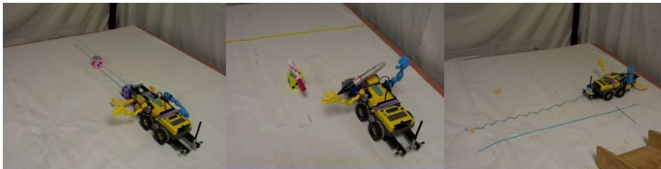
Figure 1: Robot with: (left) gripper, (middle) pen, and (right) spindle for string
