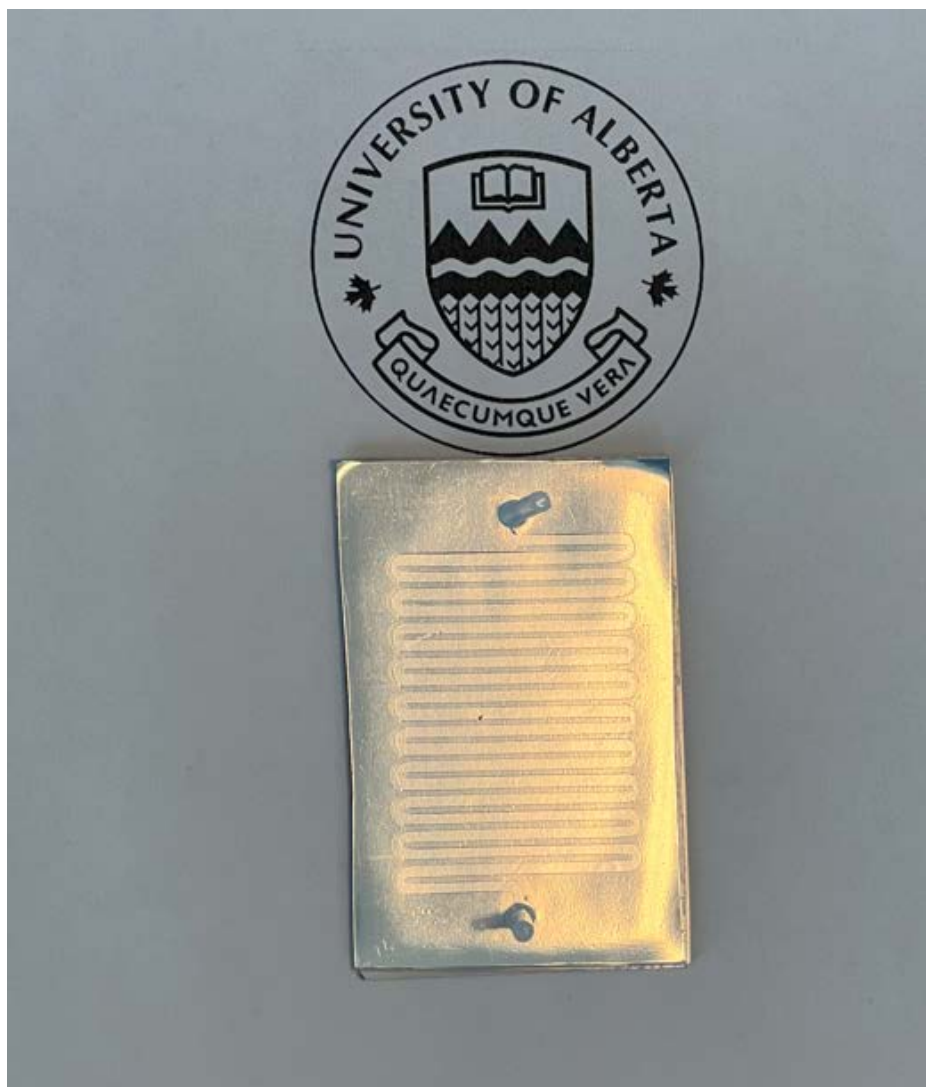
Figure S2. Shows a microfluidic device microfluidic device with an incorporated metalized sheet
