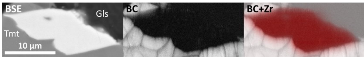
Fig. 3.2.(continued) Electron backscatter diffraction (EBSD) maps and pole figures of Group 1, 2, 3, and mixed group baddeleyite microstructures. c-d) Group 3 NWA 10299 grains 74 and 54A, showing degraded crystallinity in band contrast (BC) map despite strong BC in adjacent minerals, suggesting quasi-amorphous microstructures that diffract at length-scales below EBSD measurements. Some localized preserved baddeleyite domains with orthogonal ORs are observed in c) but diffraction is completely absent in d). Charging during EBSD analysis has resulted in slight in-run shift. BSE: backscatter electron image. IPF: inverse pole figure coloring, based on the orientation of the crystallographic z-axis. Cpx: clinopyroxene. Tmt: titanomagnetite. Gl: glass.
