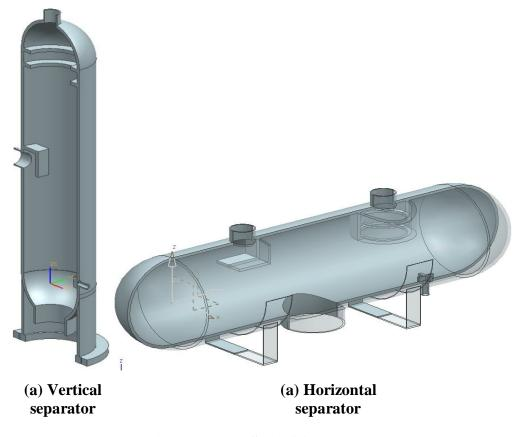
Figure 6.5: 3D Solid CAD models
