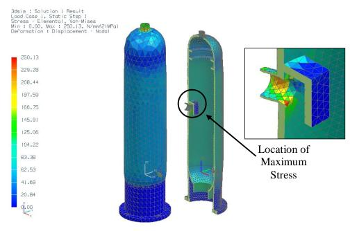
Figure 6.6: Von-Mises stress (MPa) analysis from NX Nastran for parametric 3D model of vertical separator
