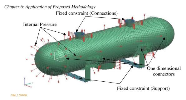
Figure 6.8: Load and constraint model
