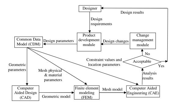
Figure 3.1: Information flow between various stages in design process
