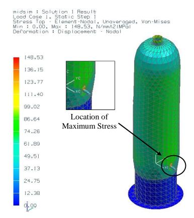
Figure 6.3: Von-Mises stress (MPa) analysis result generated from NX Nastran for parametric mid-plane model of vertical separator
