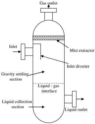
Figure A.2: Vertical Separator Layout
