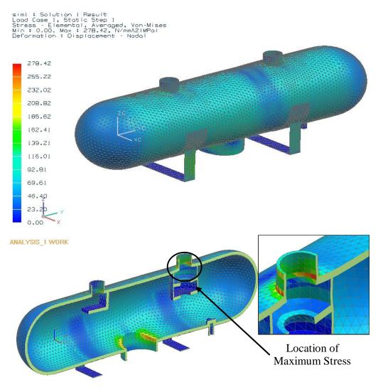
Figure 6.7: Von-Mises stress (MPa) analysis from NX Nastran for parametric 3D model of horizontal separator
