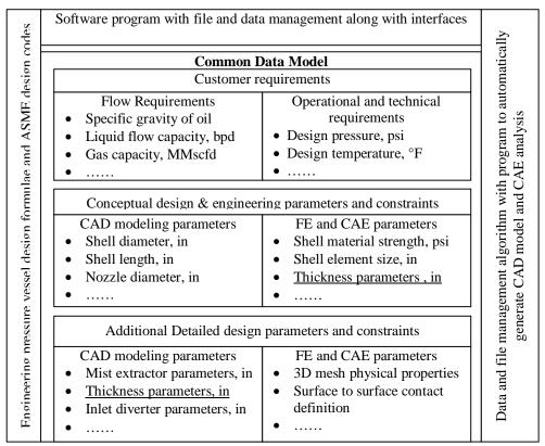
Figure 4.1: Partial CDM data for vertical separator design
