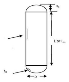
Figure A.3: Vertical separator Dimensions
