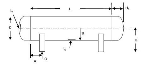
**Figure A.4: Horizontal separator Dimensions**
