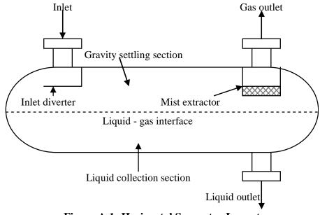
Figure A.1: Horizontal Separator Layout
