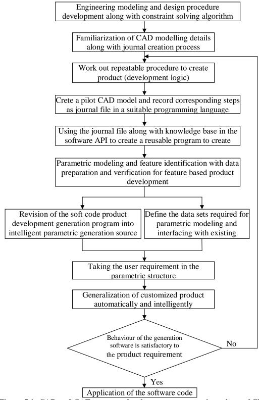
Figure 5.1: CAD and CAE program development process using a journal file
