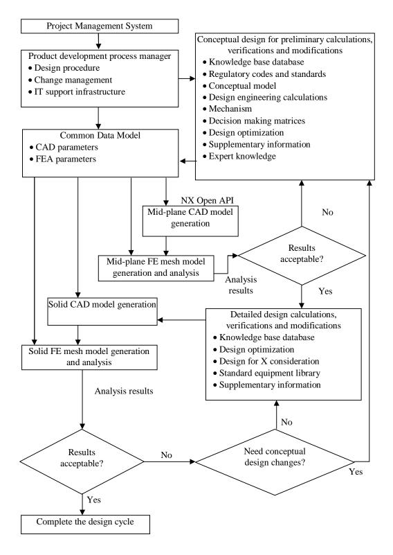
Figure 3.4: Proposed design process with CAD/CAE integration [53]
