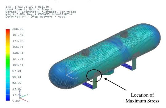
Figure 6.4: Von-Mises stress (MPa) analysis result generated from NX Nastran for parametric mid-plane model of horizontal separator
