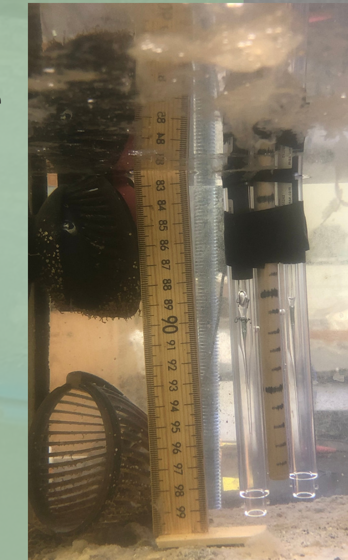
Figure 5: Unisense microsensors attached to the microsensor stand as tank depth is measured
